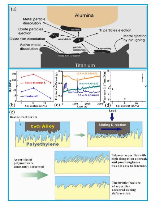
Fig. 16 (a) Tribocorrosion processes of Ti implants. Reproduced from ref. 213 with permission from Elsevier, copyright 2022. (b) Hardness *H* and elastic modulus *E*. (c) Friction coefficient curves as a function of sliding cycle. (d) Wear rate on the worn surface for the samples with 0 at% Cu, 5.2 at% Cu, and 12.6 at% Cu. Reproduced from ref. 218 with permission from Elsevier, copyright 2018. (e) Polymer surface wear model. Reproduced from ref. 219 with permission from Elsevier, copyright 2020.
