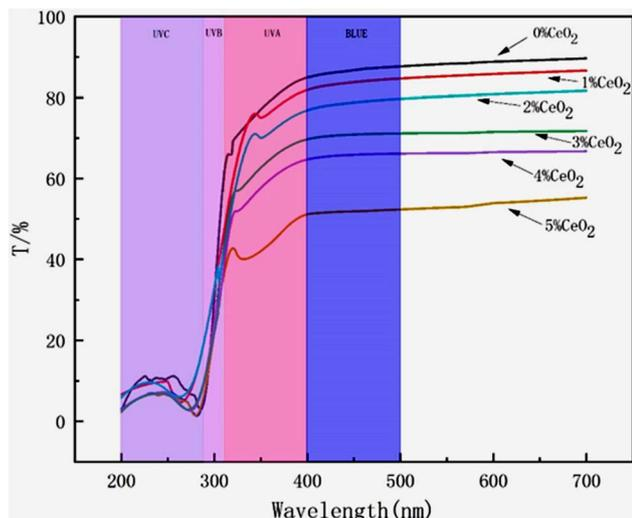
Fig. 10 UV spectral analysis of hybridized coatings.
