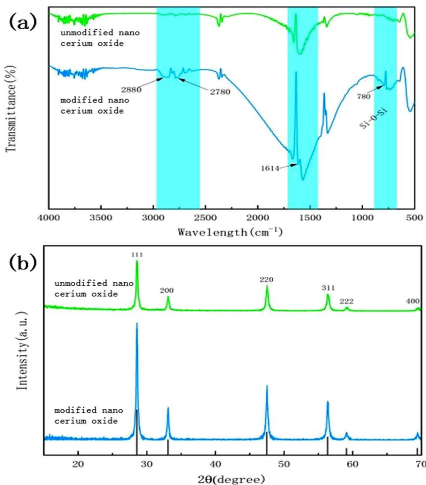
Fig. 4 (a) FTIR spectrum of n-CeO<sub>2</sub> and unmodified n-CeO<sub>2</sub> (b) X-ray pattern of n-CeO<sub>2</sub> and unmodified n-CeO<sub>2</sub>.
