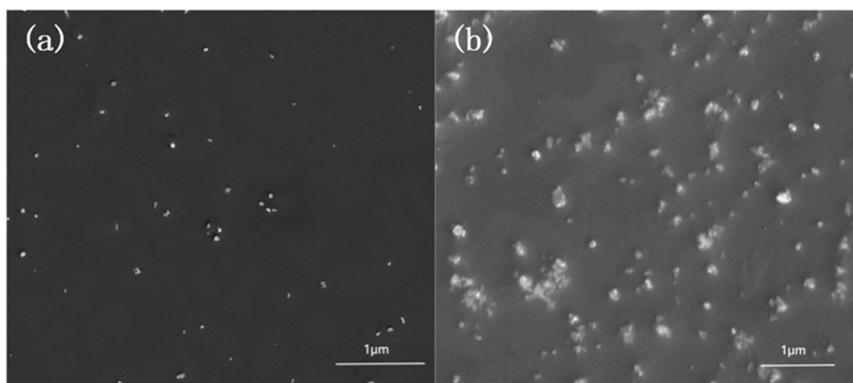
Fig. 5 (a) SEM of modified n-CeO<sub>2</sub> (b) SEM of unmodified n-CeO<sub>2</sub>.
