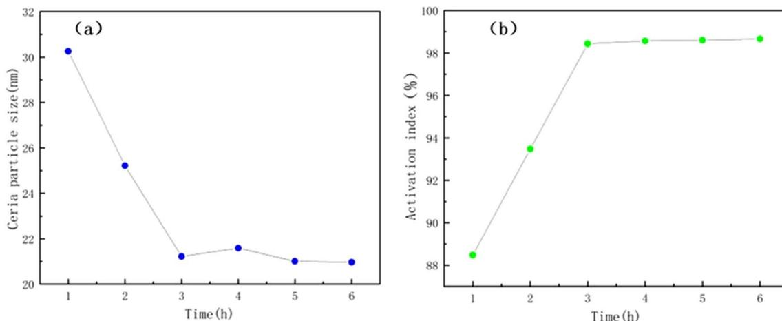
Fig. 3 Particle size analysis of modified CeO<sub>2</sub> nanoparticles at different reaction times and activation index plots (a) particle size distribution (b) activation index.
