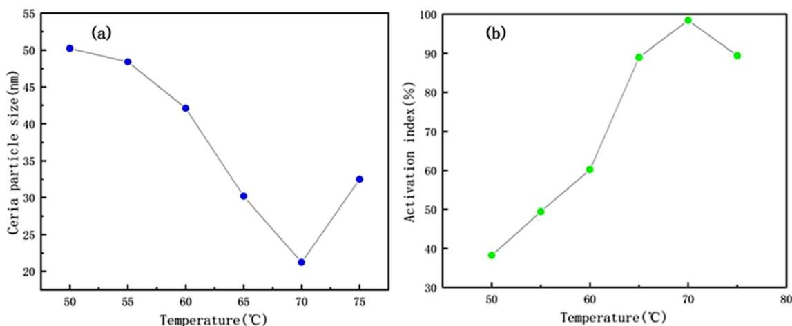
Fig. 1 Particle size analysis of modified CeO<sub>2</sub> nanoparticles at different reaction temperatures and activation index plots (a) particle size distribution (b) activation index.
