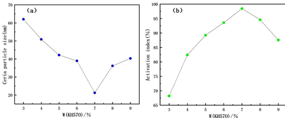
Fig. 2 Particle size analysis of modified CeO<sub>2</sub> nanoparticles with different silane coupling agent dosages and activation index plots (a) particle size distribution (b) activation index.
