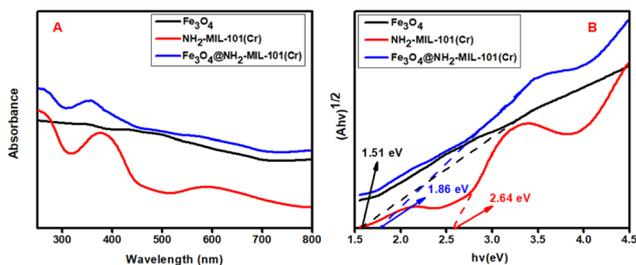
Fig. 4 UV-vis DRS (A) and Tauc plots (B) of the synthesized materials.
