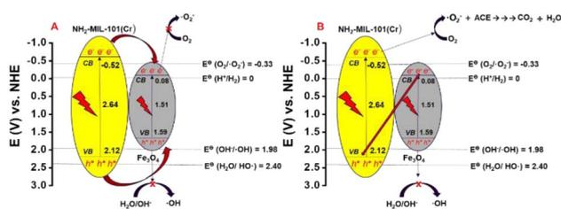
**Fig. 11** Schematic depiction of the two photocatalytic degradation mechanisms (type I (A) and Z-scheme (B) heterojunctions) of ACE over Fe<sub>3</sub>O<sub>4</sub>@NH<sub>2</sub>-MIL-101(Cr).
