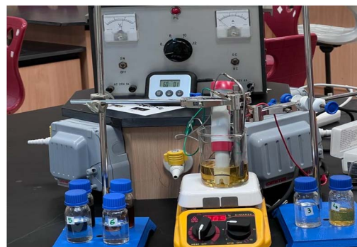
Fig. 1 The galvanostatic electrochemical setup used for paraquat degradation.
