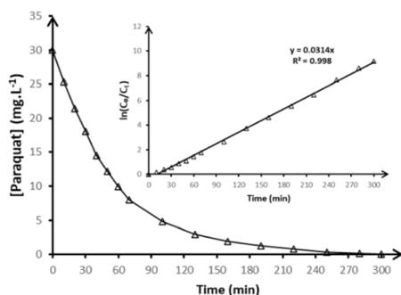
Fig. 6 Variation of the concentration of paraquat during anodic oxidation of 250 mL in 50 mmol per L  $\text{Na}_2\text{SO}_4$  in  $\text{pH} = 3$  on BDD anode at  $15 \text{ mA cm}^{-2}$  and at  $20^\circ\text{C}$ . The inset panel shows the kinetic analysis assuming a pseudo-first-order reaction.
