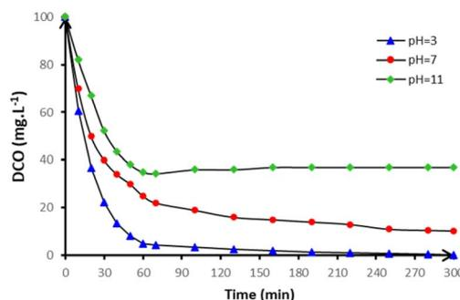
Fig. 4 Variation of chemical oxygen demand during anodic oxidation of 250 mL of  $30 \text{ mg L}^{-1}$  of paraquat in  $50 \text{ mmol per L Na}_2\text{SO}_4$  on BDD anode at  $15 \text{ mA cm}^{-2}$  and at  $20 \text{ }^\circ\text{C}$  ( $\blacktriangle$ )  $\text{pH} = 3$ , ( $\bullet$ )  $\text{pH} = 7$  and ( $\blacklozenge$ )  $\text{pH} = 11$ .
