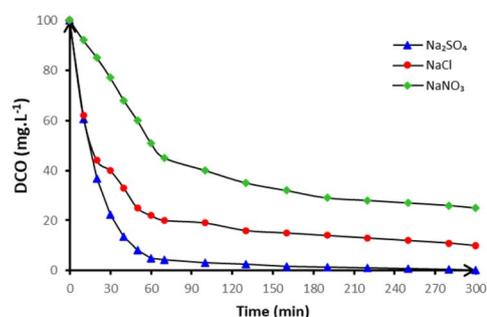
Fig. 5 Variation of chemical oxygen demand during anodic oxidation of 250 mL of  $30 \text{ mg L}^{-1}$  of paraquat in  $\text{pH} = 3$  on BDD anode at  $15 \text{ mA cm}^{-2}$  and at  $20 \text{ }^\circ\text{C}$  ( $\blacktriangle$ )  $\text{Na}_2\text{SO}_4$ , ( $\bullet$ ) NaCl and ( $\blacklozenge$ )  $\text{NaNO}_3$ .
