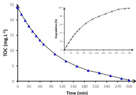
Fig. 8 TOC removal with time during anodic oxidation of 250 mL of 30 mg L<sup>-1</sup> of paraquat in 50 mmol per L Na<sub>2</sub>SO<sub>4</sub> in pH = 3 on BDD anode at 15 mA cm<sup>-2</sup> and at 20 °C. The inset shows the degradation %.
