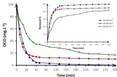
Fig. 3 Influence of applied current density on the evolution of DCO during anodic oxidation of 250 mL of  $30 \text{ mg L}^{-1}$  of paraquat in  $50 \text{ mmol per L Na}_2\text{SO}_4$  at  $\text{pH} = 3.0$  and at  $20 \text{ }^\circ\text{C}$  on BDD anode, ( $\blacklozenge$ )  $10 \text{ mA cm}^{-2}$ , ( $\blacktriangle$ )  $15 \text{ mA cm}^{-2}$  and ( $\bullet$ )  $20 \text{ mA cm}^{-2}$ . The inset shows the removal %.
