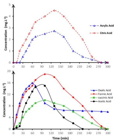
Fig. 11 Time-course of the concentration of relevant carboxylic acids detected during anodic oxidation of 250 mL in 50 mmol per L  $\text{Na}_2\text{SO}_4$  in pH = 3 on BDD anode at  $15 \text{ mA cm}^{-2}$  and at  $20 \text{ }^\circ\text{C}$ .
