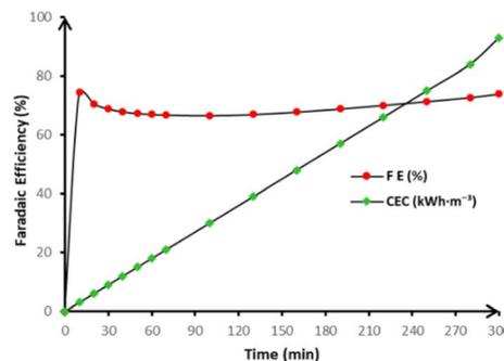
Fig. 7 Variation of faradaic efficiency ( $\blacktriangle$ ) and energy consumption ( $\square$ ) during anodic oxidation of 250 mL in 50 mmol per L  $\text{Na}_2\text{SO}_4$  in  $\text{pH} = 3$  on BDD anode at  $15 \text{ mA cm}^{-2}$  and at  $20^\circ\text{C}$ .
