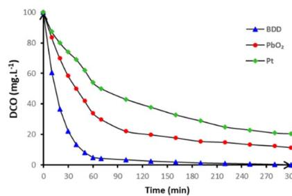
Fig. 2 Variation of chemical oxygen demand during anodic oxidation of 250 mL of 30 mg L<sup>-1</sup> of paraquat in 50 mmol per L Na<sub>2</sub>SO<sub>4</sub> at pH = 3.0 (▲) BDD, (●) PbO<sub>2</sub> and (◆) Pt anodes and a graphite cathode operating at 15 mA cm<sup>-2</sup> and at 20 °C.
