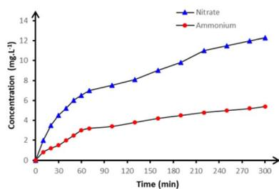
Fig. 12 Accumulation of nitrate ( $\blacktriangle$ ) and ammonium ( $\bullet$ ) ions detected during anodic oxidation of 250 mL in 50 mmol per L  $\text{Na}_2\text{SO}_4$  in pH = 3 on BDD anode at  $15 \text{ mA cm}^{-2}$  and at  $20 \text{ }^\circ\text{C}$ .
