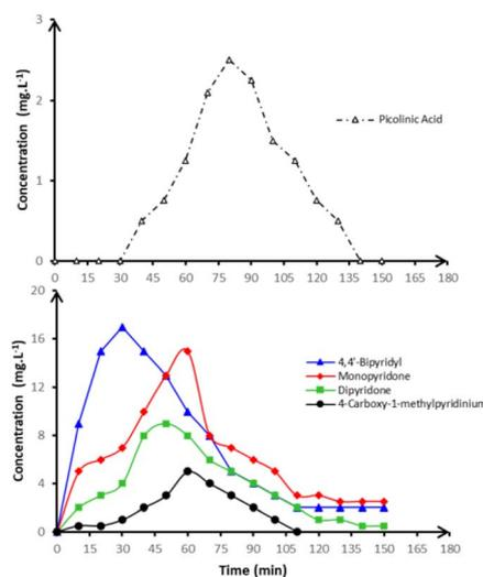
Fig. 10 Time evolution of paraquat and its aromatic degradation intermediates detected during anodic oxidation of 250 mL in 50 mmol per L  $Na_2SO_4$  in pH = 3 on BDD anode at  $15 \text{ mA cm}^{-2}$  and at  $20^\circ \text{C}$ .
