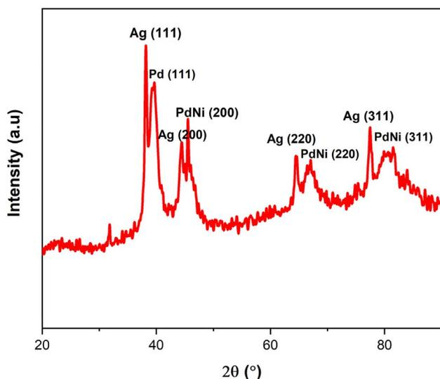
Fig. 1 XRD pattern of PdNiAg NPs.
