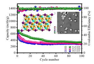
Fig. 2 Reversible capacity of FLaN-MOF after 100 cycles at  $100~\mathrm{mA~g^{-1}}$ . Reproduced from ref. 35 with permission from Elsevier, copyright 2021.
