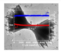
Fig. 5 Capacitance of  $CeO_2$  electrode material after 10 000 cycles. Reproduced from ref. 52 with permission from Elsevier, copyright 2016.
