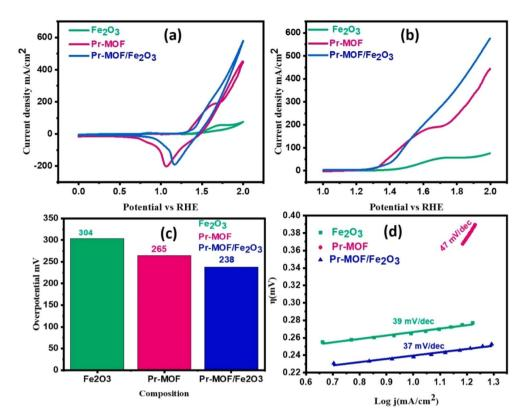
Fig. 7 (a) Cyclic voltammograms; (b) linear scanning voltammograms; (c) comparison of overpotentials at a current density of 10 mA cm $^{-2}$ ; and (d) Tafel slopes for Fe<sub>2</sub>O<sub>3</sub>, Pr-MOF, and Pr-MOF/Fe<sub>2</sub>O<sub>3</sub>. Reproduced from ref. 65 with permission from Elsevier, copyright 2023.
