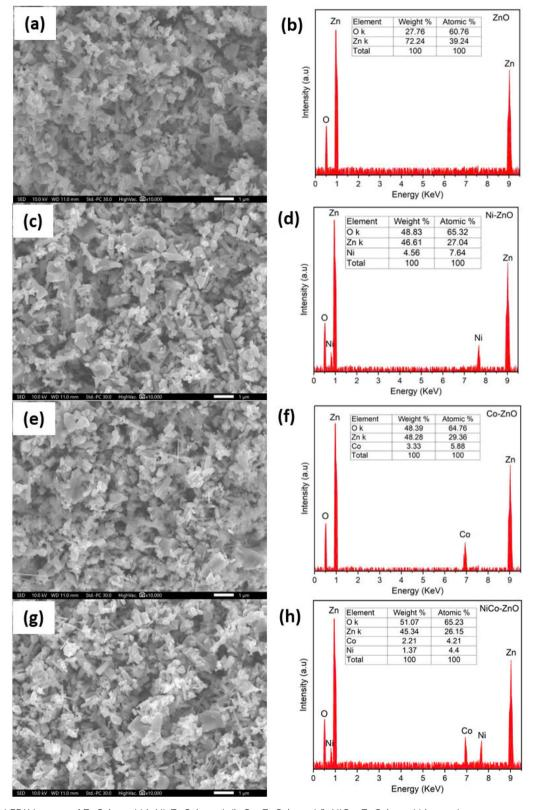
Fig. 11 SEM and EDX images of ZnO (a and b), Ni-ZnO (c and d), Co-ZnO (e and f), NiCo-ZnO (g and h) samples.
