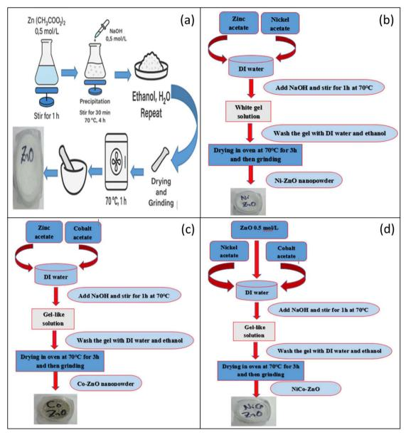
Schematic representation of the synthesis steps: (a) ZnO, (b) Ni-ZnO, (c) Co-ZnO, (d) NiCo-ZnO.
