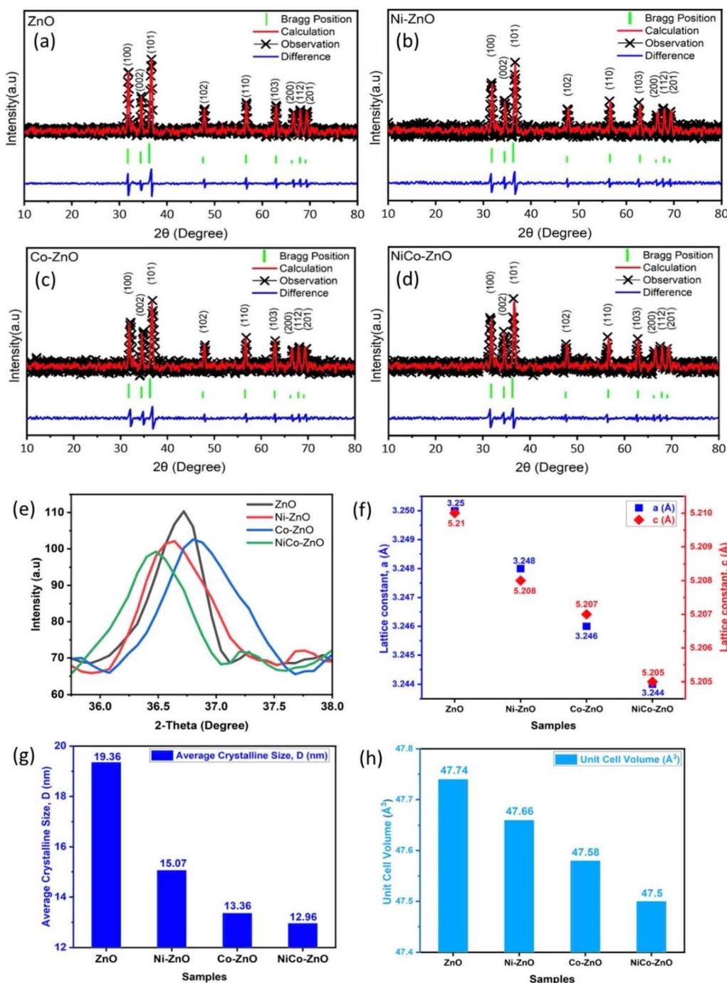
Fig. 8 Rietveld refinement plots of ZnO (a), Ni-ZnO (b), Co-ZnO (c), NiCo-ZnO (d); peak broadening comparison of (101) planes for the nanomaterials (e); lattice constants (*a*, *c*) of samples (f); crystallite size comparison among the nanomaterials (g); unit cell volume comparison among the nanomaterials (h).
