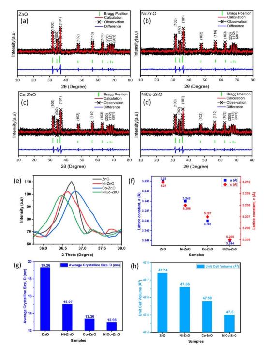
Fig. 8 Rietveld refinement plots of ZnO (a), Ni-ZnO (b), Co-ZnO (c), NiCo-ZnO (d); peak broadening comparison of (101) planes for the nanomaterials (e); lattice constants (a, c) of samples (f); crystallite size comparison among the nanomaterials (g); unit cell volume comparison among the nanomaterials (h).
