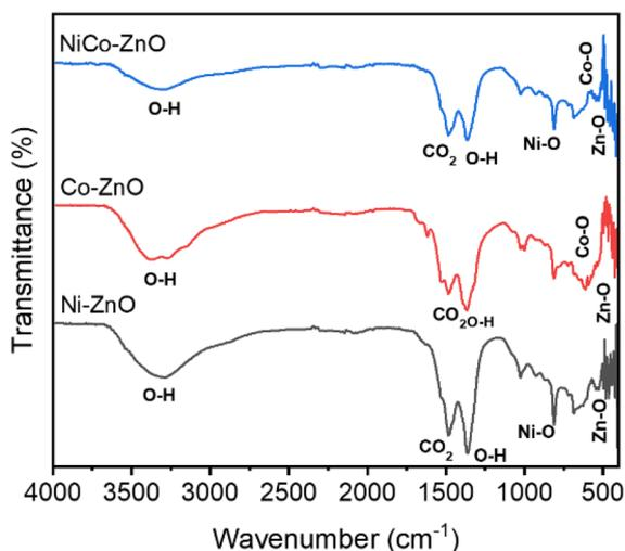
Fig. 9 FTIR spectra of Ni-ZnO (black line), Co-ZnO (red line), NiCo-ZnO (blue line) samples.
