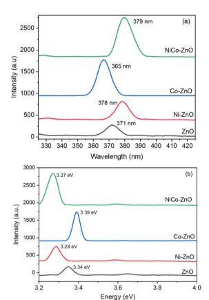
Fig. 10 Photoluminescence emission (a) and bandgap spectra (b) for ZnO, Co-ZnO, Ni-ZnO, and NiCo-ZnO
