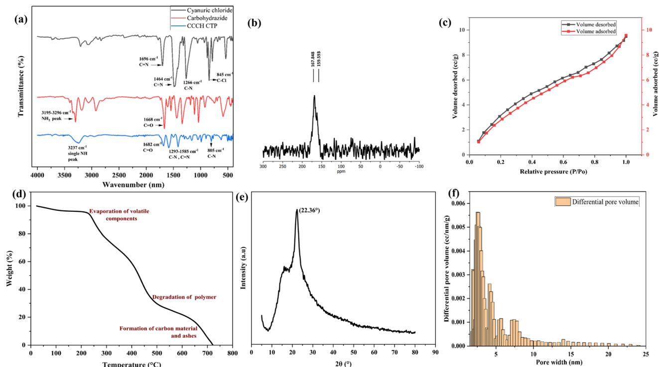
Fig. 3 (a) FT-IR spectrum for reactants and polymer CCCH CTP, (b)  $^{13}\text{C}$  CPMAS NMR spectrum, (c) nitrogen sorption isotherm, (d) TGA curve, (e) XRD pattern, (f) pore size distribution curve for CCCH CTP.
