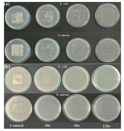
Fig. 6 Antibacterial test results of (a) Cu-based TENG and (b) C5P5-based TENG at different operation times: 0, 30, 60 and 120 seconds.
