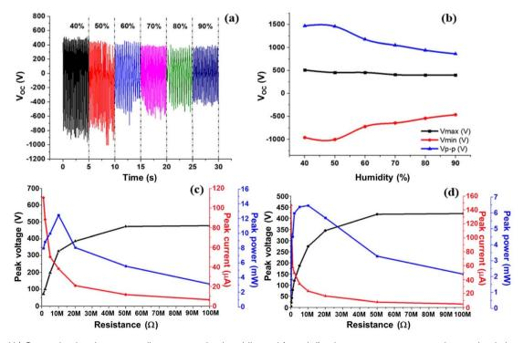
Fig. 5 (a and b) Open-circuit voltage according to operating humidity and (c and d) volt-ampere-power vs. resistance load characteristics at 40% and 90% humidity of C5P5-based TENG.
