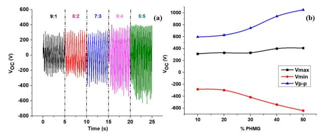
Fig. 4 (a) Open-circuit voltage  $V_{OC}$  output and (b) the  $V_{OC}$  profiles of TENG devices with CS-PHMG-GA electrodes prepared at various PHMG-GA/CS mass ratios under 70% RH.
