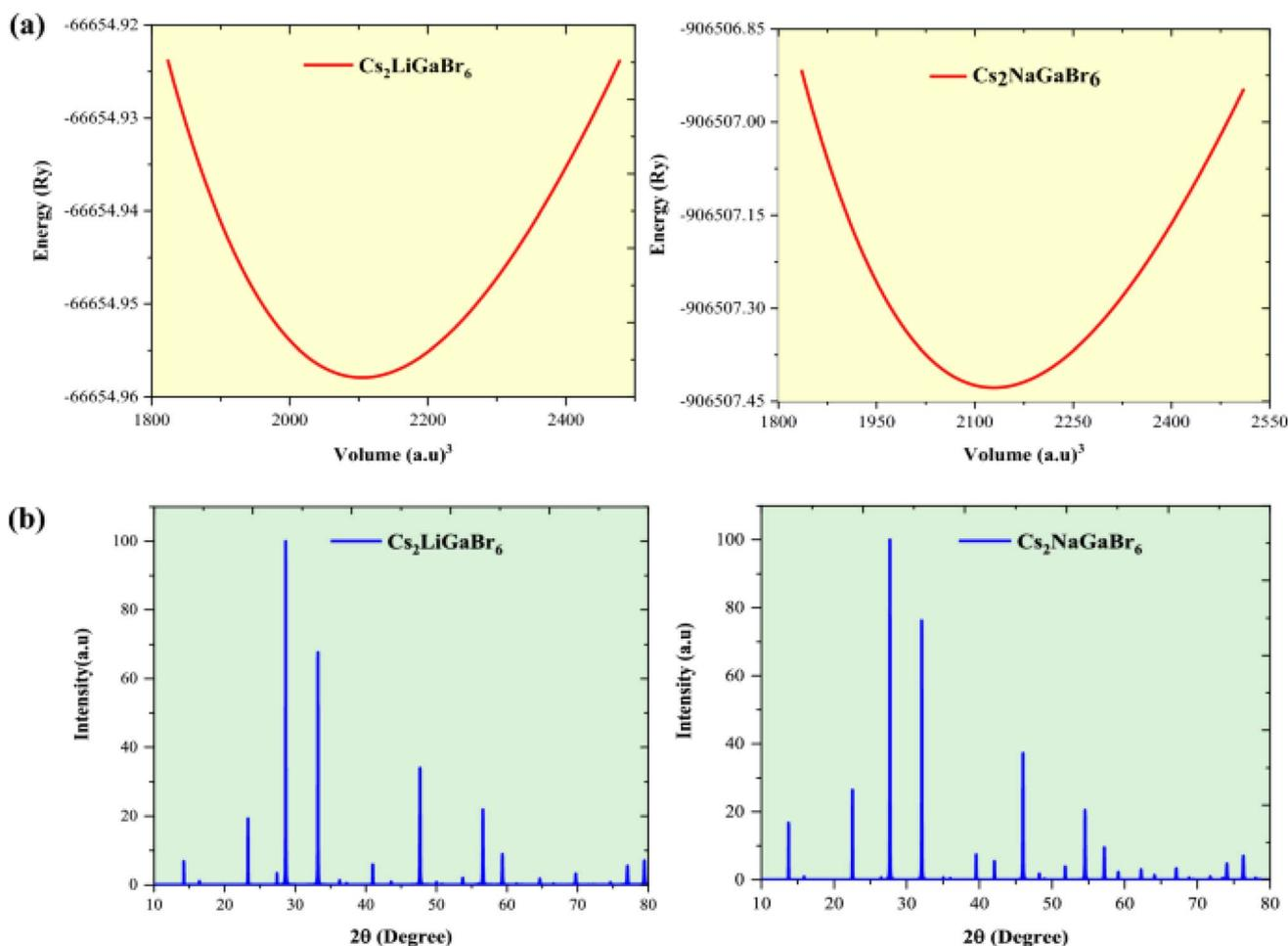
Fig. 6 (a) Graphical depiction of the optimized volume–energy relationship, and (b) DFT-simulated XRD patterns of  $\text{Cs}_2\text{MGA}_6$  ( $M = \text{Li}, \text{Na}$ ) double halide perovskites.<sup>199</sup>
