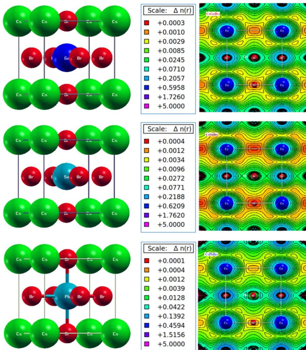
Fig. 16 The crystal structure and electronic charge density in (100) plane of the unit cells for metal halide perovskites  $\text{CsNBr}_3$  ( $\text{N}^{2+} = \text{Ge, Sn, Pb}$ ), in cubic symmetry (space group  $Pm\bar{3}m$ ; IT No. 221) optimized using GGA approaches. Color legend: cesium (green), germanium (dark Blue), tin (sky blue) and lead (steel blue), and bromine (red).<sup>212</sup>
