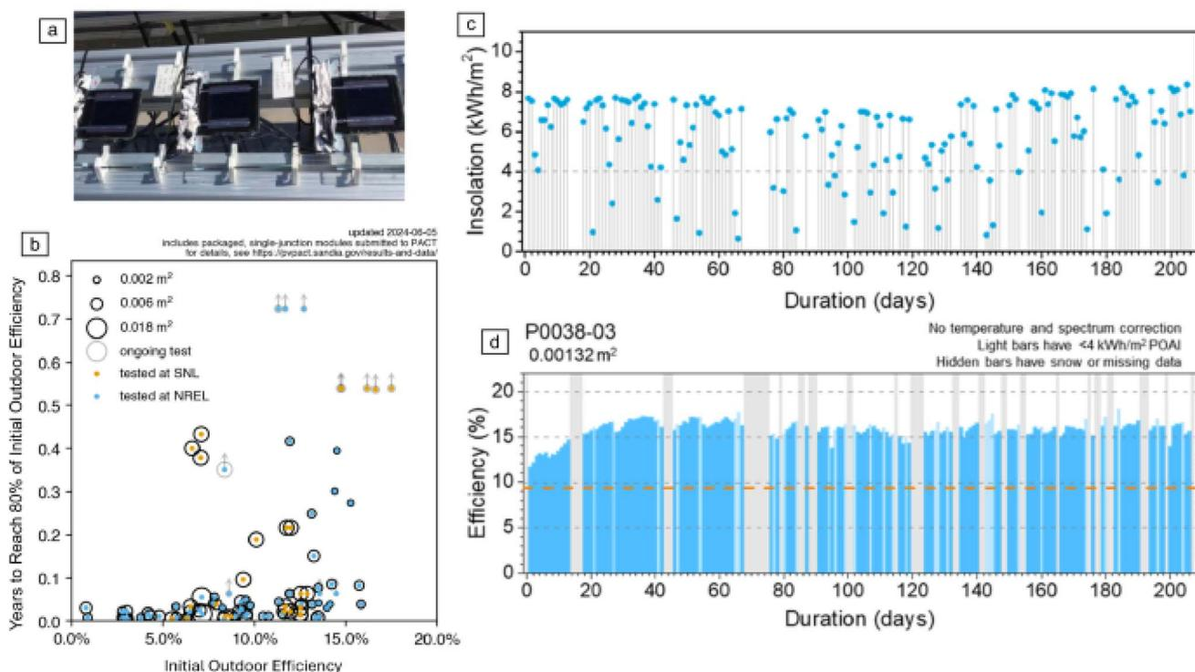
Fig. 10 Outdoor field stability test results. Pictures of modules installed outdoor (a). Outdoor stability test results at the perovskite PV Accelerator for Commercializing Technologies (PACT) (b). SNL, Sandia National Laboratories; NREL, National Renewable Energy Laboratory. Light intensity (c) and resulting device performance of one of the modules at PACT (d).<sup>203</sup>
