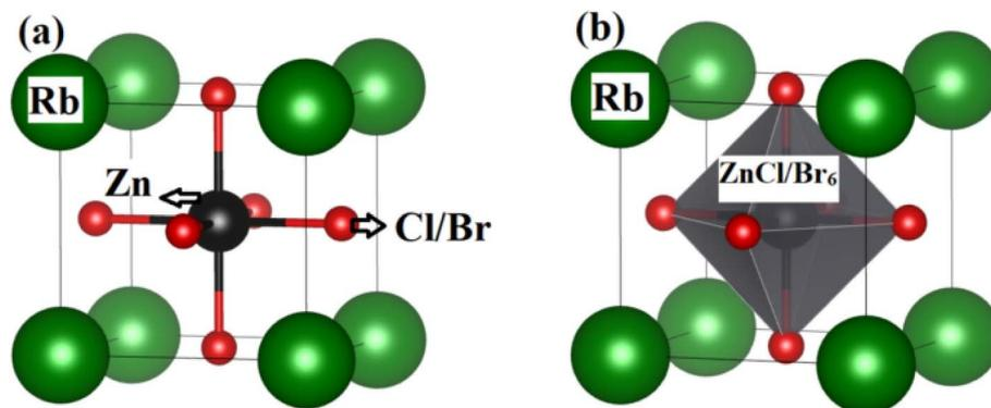
Fig. 5 (a) Crystal structure (b) octahedra of  $\text{ZnCl}_6/\text{Br}_6$  of  $\text{RbZnX}_3$  ( $\text{X} = \text{Cl}, \text{Br}$ ) perovskites.<sup>198</sup>
