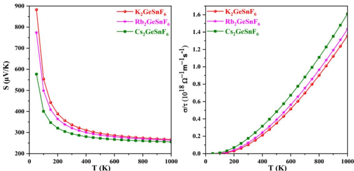
Fig. 13 Variation of electrical conductivity and seebeck coefficient with temperature for  $\text{A}_2\text{GeSnF}_6$  ( $A = \text{K}, \text{Rb}, \text{Cs}$ ).<sup>210</sup>
