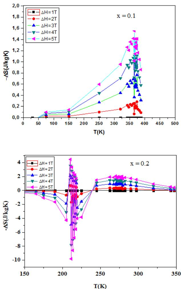
Fig. 8 Variation of the magnetic entropy as a function of the temperature and the magnetic field of the compounds  $\text{La}_{1-x}\text{Ag}_x\text{SrMn}_2\text{O}_{5+\delta}$  ( $x = 0.1$  and  $x = 0.2$ ).
