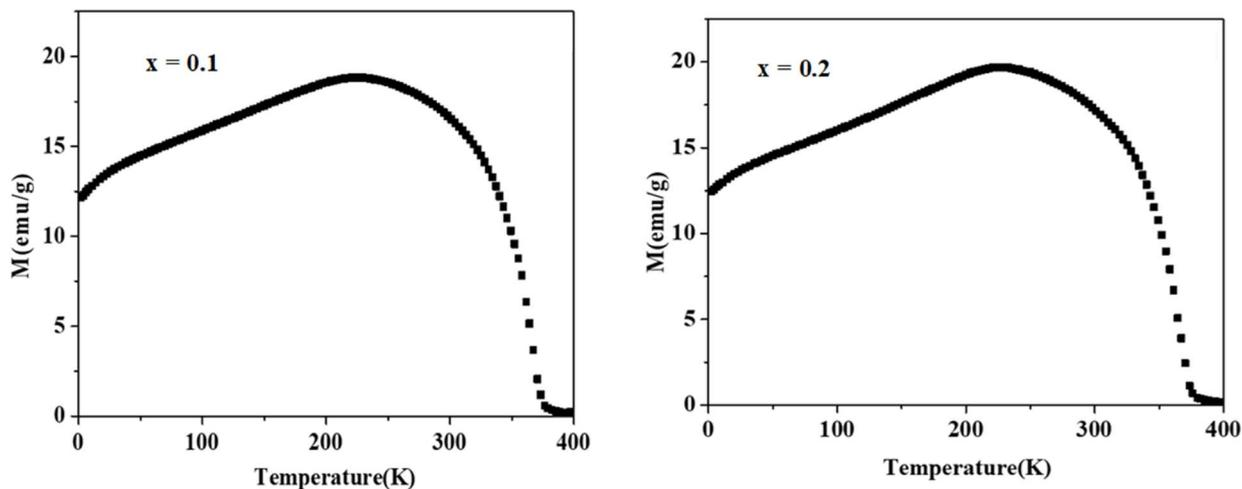
Fig. 4 Variation of the magnetization as a function of temperature for  $x = 0$ ,  $x = 0.1$  and  $x = 0.2$ .
