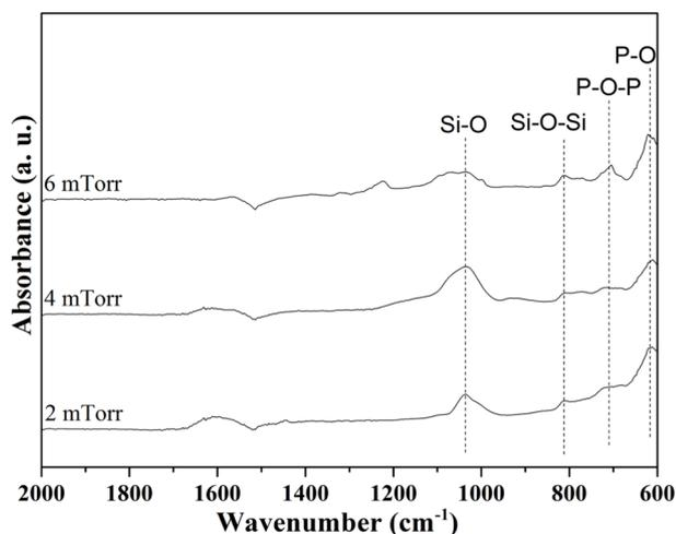
Fig. 6 FTIR spectra of thin film BG specimens with working pressures of 2 mTorr, 4 mTorr, and 6 mTorr after SBF immersion for 14 d.
