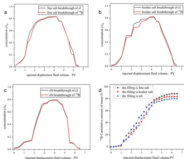
Fig. 7 Breakthrough curves of  $^{10}\text{B}$  tracer and  $\text{Cl}^-$  in porous media: (a) fine salt; (b) kosher salt; (c) silt; (d) effluent concentration versus injected pore volume across packing materials.
