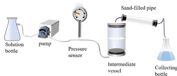
Fig. 1 Schematic diagram of the mobility experimental setup.
