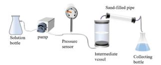
Fig. 1 Schematic diagram of the mobility experimental setup.
