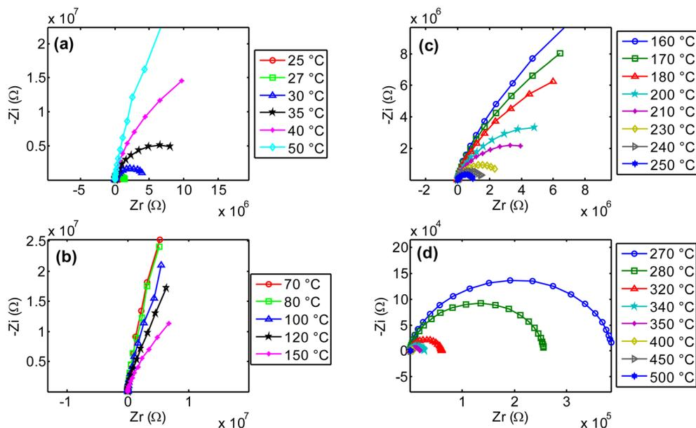
Fig. 17 Nyquist plots of NdCaFeSnO<sub>6</sub> impedance in several range of temperatures.
