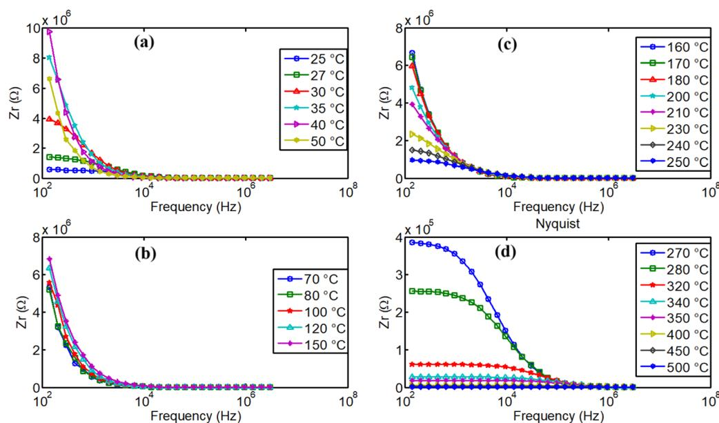
Fig. 16 Impedance dispersion of real part of impedance in  $\text{NdCaFeSnO}_6$  ceramics.
