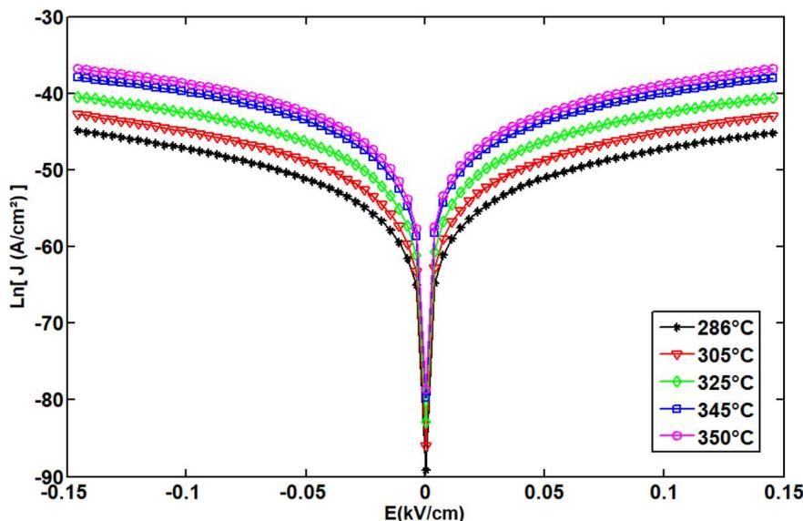
Fig. 22 Diode like conduction mechanism in the NdCaFeSnO<sub>6</sub> ceramic.
