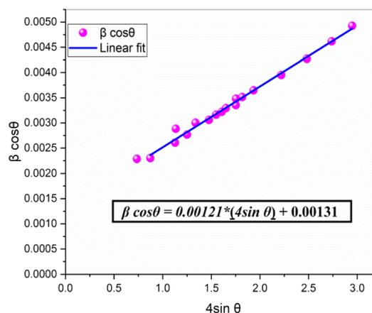
**Fig. 5** Williamson–Hall plot for estimating the crystallite size and lattice strain of the NdCaFeSnO<sub>6</sub> compound. The slope represents the lattice strain ( $\varepsilon$ ), while the y-intercept provides an estimate of the crystallite size ( $D$ ).
