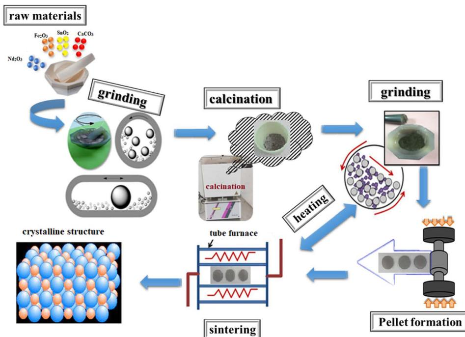
Fig. 1 Schematic description of the elaboration process of NdCaFeSnO<sub>6</sub> ceramics *via* the solid-state method.
