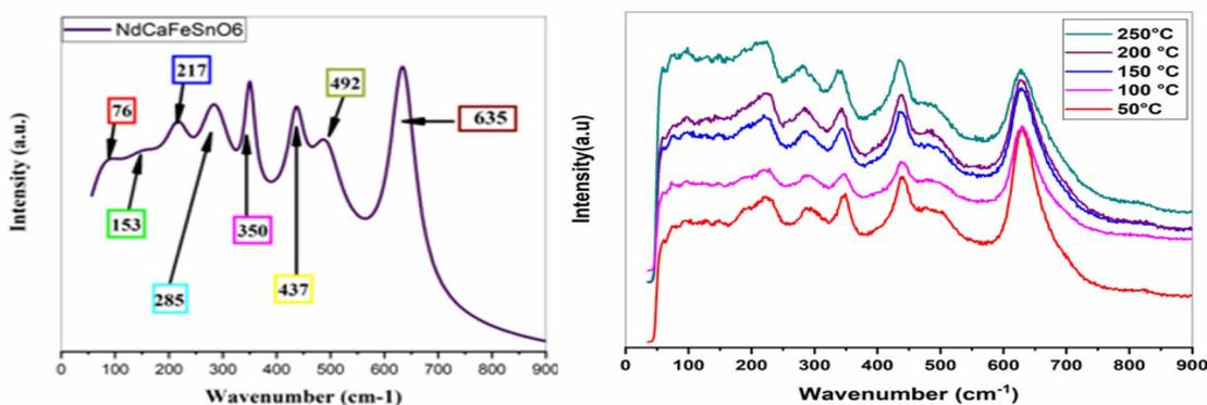
Fig. 9 Room temperature Raman spectra of NdCaFeSnO<sub>6</sub> sample.
