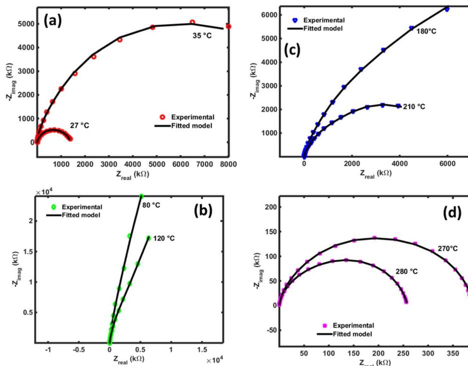
Fig. 19 Experimental and fitted curves of NdCaFeSnO<sub>6</sub> impedance spectral responses in Nyquist plots for some temperatures chosen in the 3 regions.
