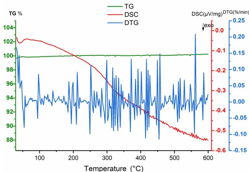
Fig. 15 Thermal analysis results obtained from  $\text{NdCaFeO}_6$  ceramic. The thermogravimetric (TGA, green curve) signal shows flat curve indicating mass stability. Differential Scanning Calorimetry (DSC, red curve) displays uniform variation related to grain reordering *versus* temperature. The derivative thermogravimetry (DTG, blue curve) highlights almost weak variation of the mass.
