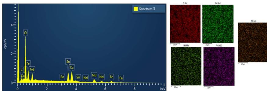
Fig. 8 EDX spectrum of NdCaFeSnO<sub>6</sub> compound.
