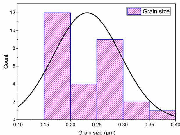
Fig. 7 Histogram of the grain size distribution for NdCaFeSnO<sub>6</sub>.
