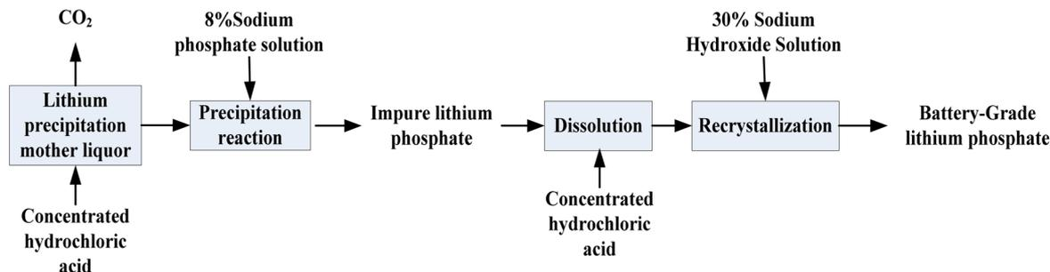
Fig. 10 Process flow diagram for lithium phosphate preparation.
