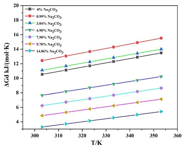
Fig. 9 Plot of the Gibbs free energy ( $\Delta G_d$ ) change versus temperature.
