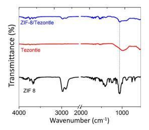
Fig. 5 FTIR spectra of the pristine supports with their respective functional groups (Tables 1 and 2).
