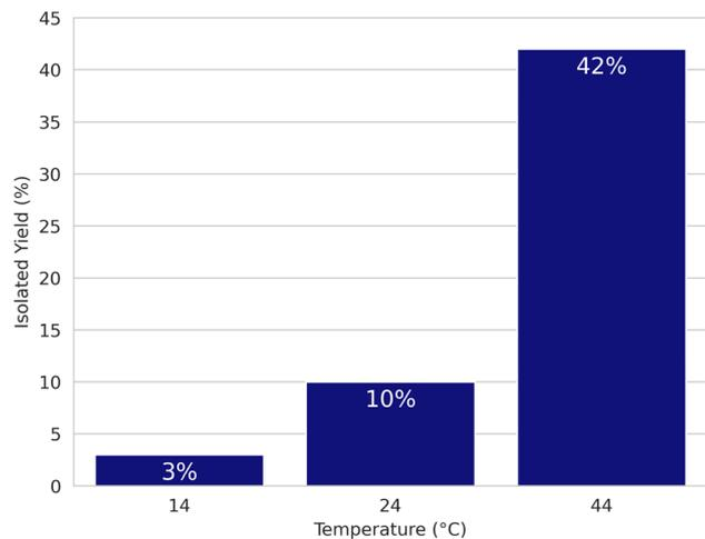
Fig. 2 Temperature influence on isolated yield of 7. Reaction termination was determined based on full consumption of starting material via  $^1\text{H}$  NMR. The time to achieve conversion was determined to be 144, 91, and 66 hours (Left to Right).
