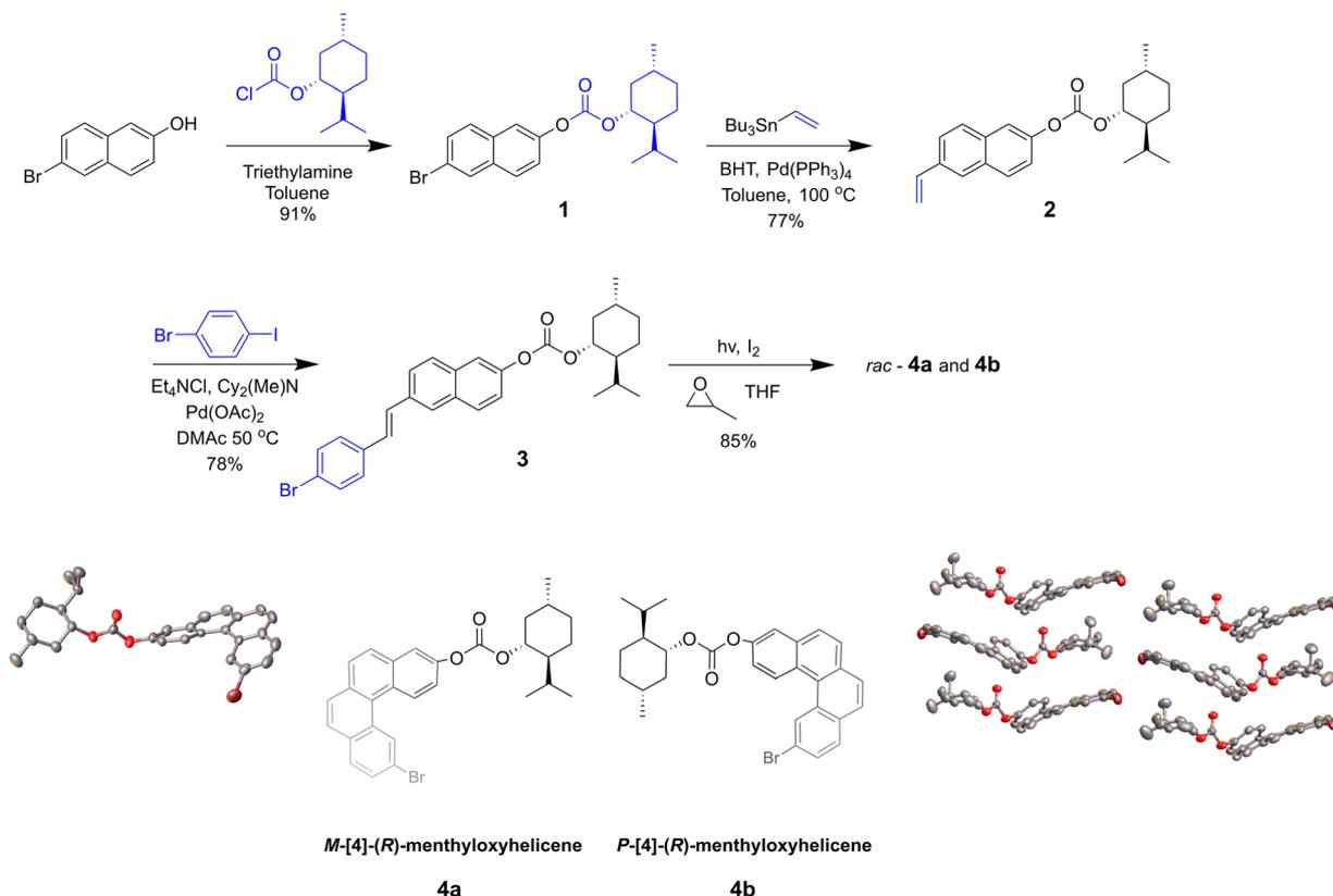
**Scheme 1** Synthesis of *rac*-[4]-menthyloxycarbonato-helicene accompanied by crystal structure (left) and its packing (right). Racemic mixture is labeled from the standpoint of *P* and *M*-[4]-helicene, ignoring stereochemistry of the menthyloxycarbonato group. Butylated hydroxytoluene is abbreviated as BHT.
