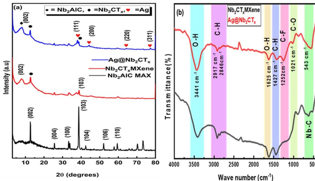
Fig. 2 (a) XRD spectra of  $\text{Nb}_2\text{AlC}$  MAX (black),  $\text{Nb}_2\text{CT}_x$  MXene (red),  $\text{Ag@Nb}_2\text{CT}_x$  ( $\text{C}_2$ ) (blue), (b) FTIR spectra of  $\text{Nb}_2\text{CT}_x$  MXene, and  $\text{Ag@Nb}_2\text{CT}_x$  ( $\text{C}_2$ ). The figure should be in high magnification.
