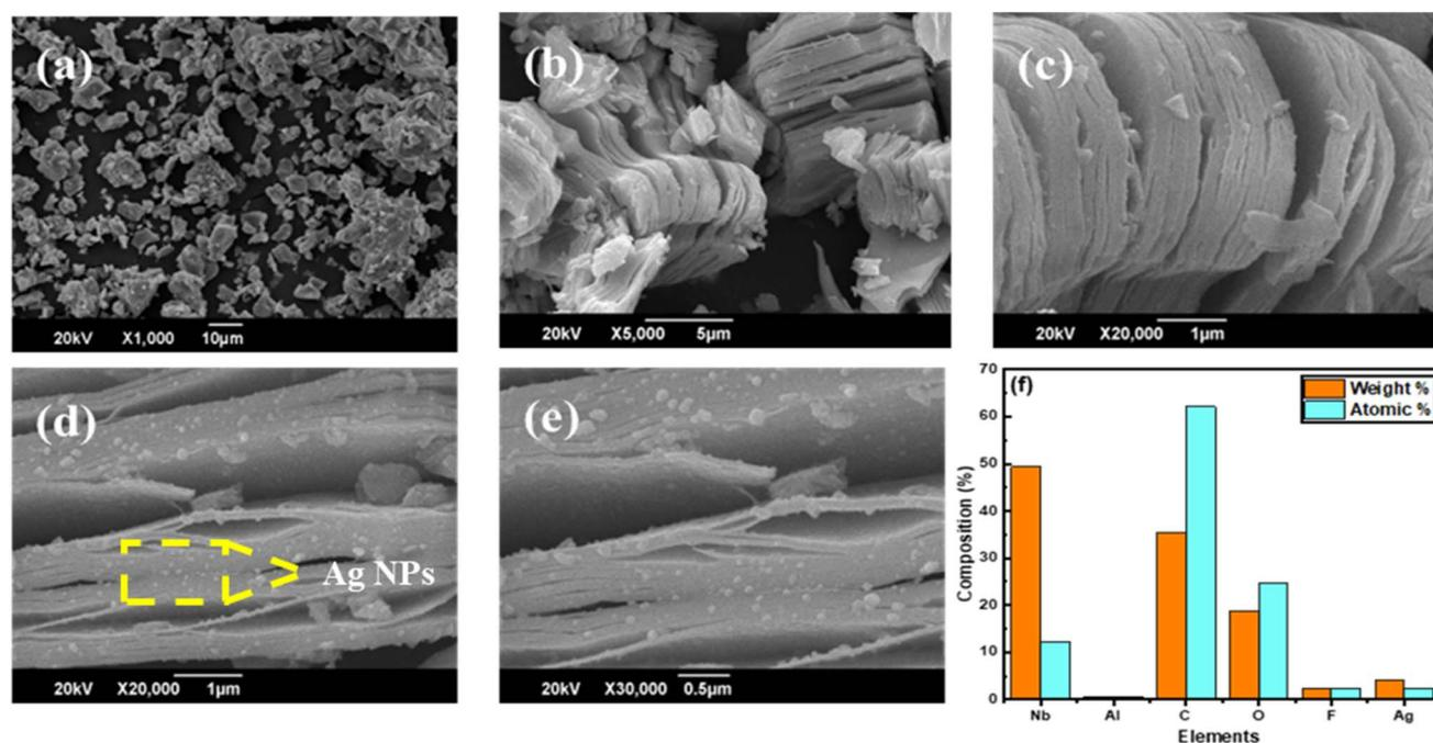
Fig. 4 SEM images of (a)  $\text{Nb}_2\text{AlC}$  MAX, (b and c) pristine  $\text{Nb}_2\text{CT}_x$  MXene, (d and e)  $\text{Ag}@\text{Nb}_2\text{CT}_x$  ( $\text{C}_2$ ), (f) EDX plot for the elemental analysis of  $\text{Ag}@\text{Nb}_2\text{CT}_x$ .
