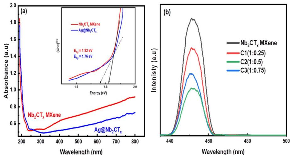
Fig. 6 (a) Absorbance and band gap of pristine  $\text{Nb}_2\text{CT}_x$  MXene and  $\text{Ag}@\text{Nb}_2\text{CT}_x$  ( $\text{C}_2$ ), (b) Photoluminescence (PL) spectra of pristine MXene and nanocomposites.
