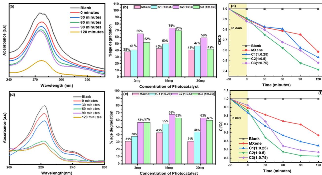
Fig. 5 (a and d) Absorbance spectra of Ag@Nb<sub>2</sub>CT<sub>x</sub> (C<sub>2</sub>) showing the degradation efficiency of norfloxacin and feroxacin antibiotics from solutions at different times respectively, (b and e) comparison of different photocatalysts at various ratios, (c and f) photocatalytic degradation of norfloxacin and feroxacin antibiotics in the presence of pristine MXene and nanocomposites.
