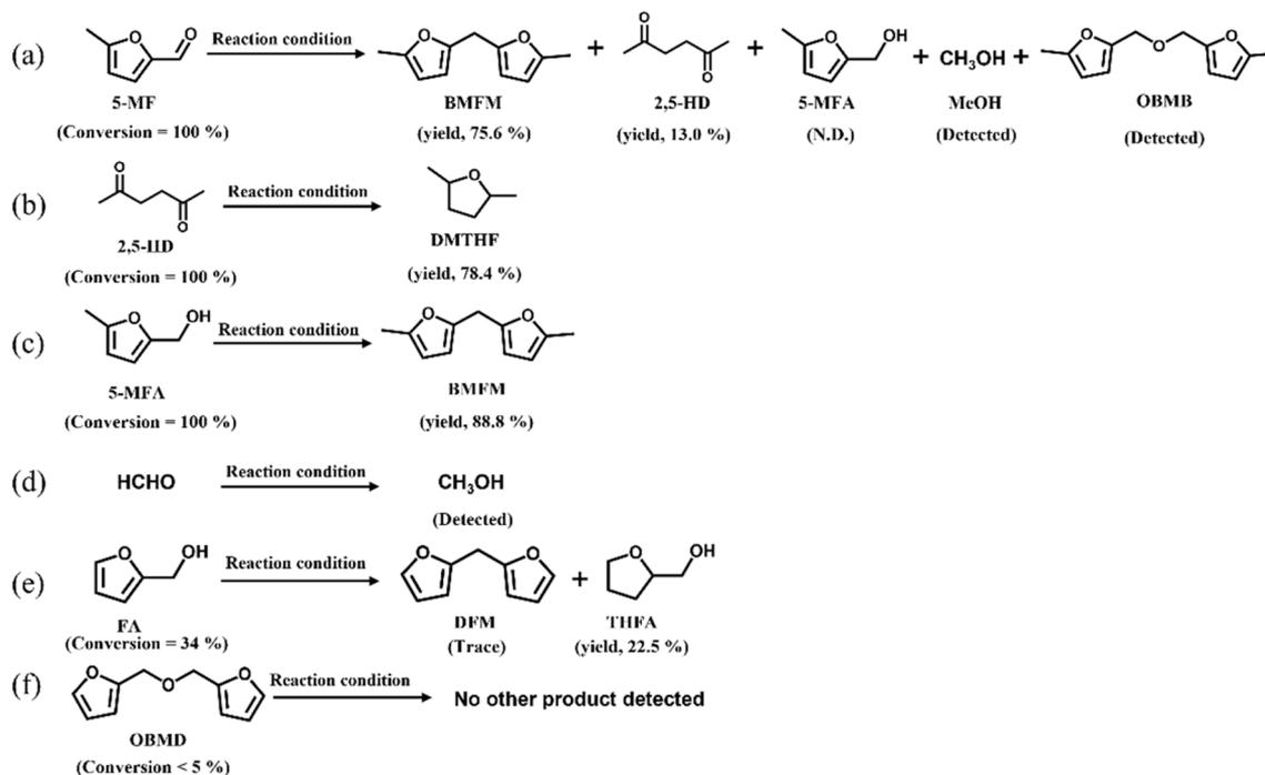
Scheme 2 Control experiments. Reaction conditions: substrate (1 mmol), RuCu/HAP (50 mg), cyclohexane (5 mL) and water (5 mL), 100 °C, H<sub>2</sub> (4 MPa), 4 h.
