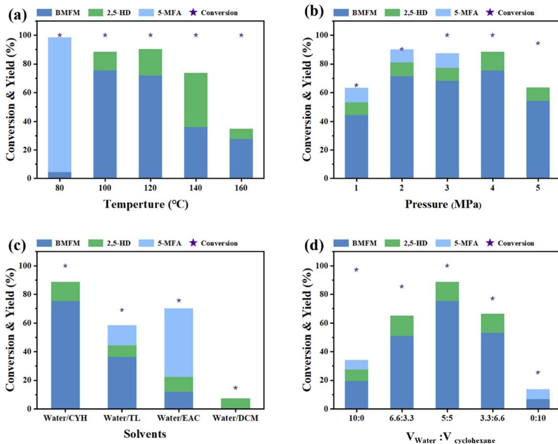
Fig. 1 Effect of (a) reaction temperatures, (b) hydrogen pressures (reaction conditions: 1 mmol 5-MF, 50 mg RuCu/HAP,  $V_{\text{cyclohexane}} : V_{\text{water}} = 1 : 1$ ),  $\text{H}_2$  (4 MPa), 4 h. Effect of (c) organic solvents types and (d) the volume proportion of cyclohexane.
