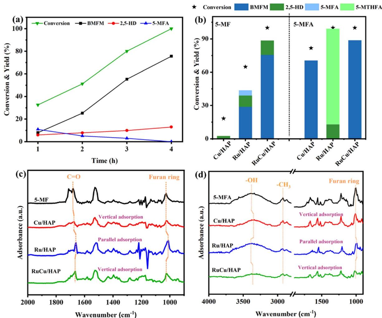
Fig. 5 (a) 5-MF conversion and products yield at different reaction times, reaction conditions: 5-MF (1 mmol), catalyst (50 mg), cyclohexane (5 mL) and water (5 mL), 100 °C, H<sub>2</sub> (4 MPa), 4 h. (b) Conversion of 5-MFA with different catalysts. (c) ATR-IR spectra of 5-MF adsorbed over catalysts; (d) ATR-IR spectra of 5-MFA adsorbed over catalysts.
