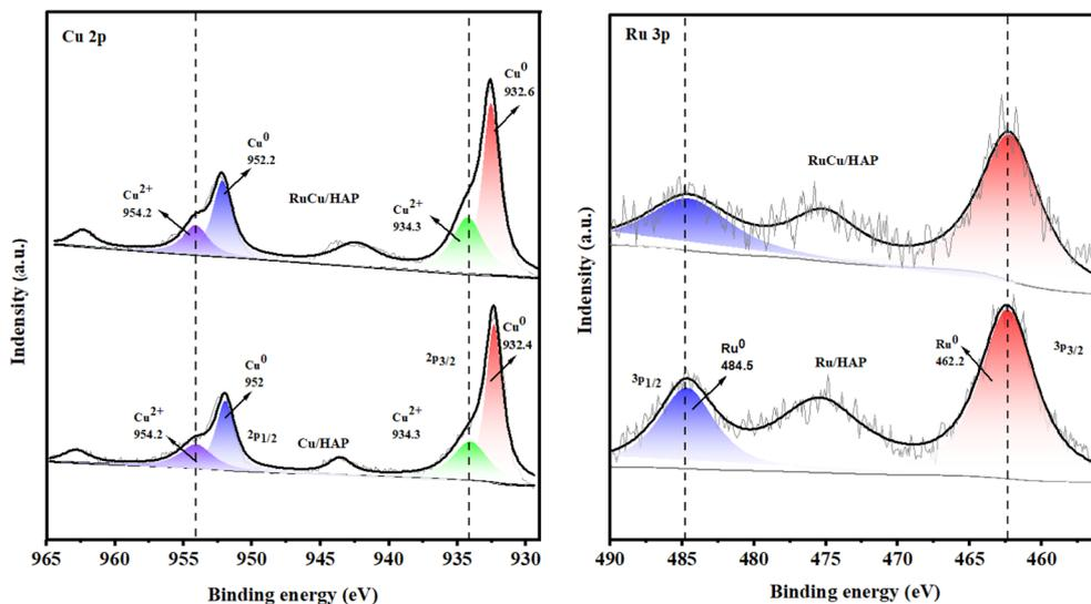
Fig. 4 High-resolution XPS of the monometallic and bimetallic catalysts for (a) Cu 2p<sub>3/2</sub>, (b) Ru 3p<sub>3/2</sub>.
