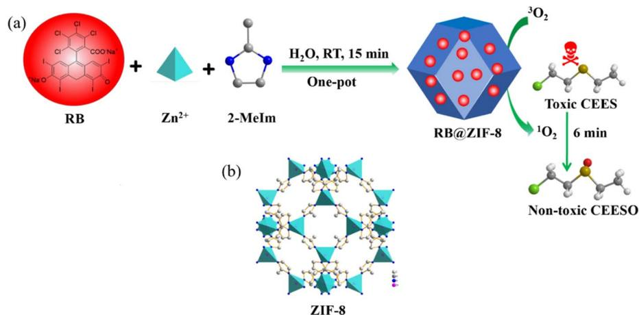
**Scheme 1** (a) The synthesis process of RB@ZIF-8 composite and its application as a visible light-driven heterogeneous photosensitizer for the efficient detoxification of a sulfur mustard simulant in air. (b) The crystal structure of ZIF-8.
