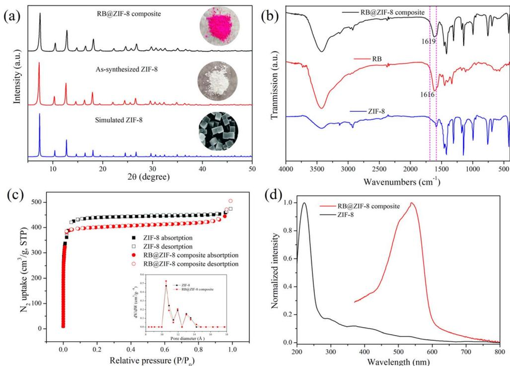
Fig. 1 (a) PXRD patterns of RB@ZIF-8 composite, as-synthesized ZIF-8 and simulated ZIF-8. The photographs of RB@ZIF-8 composite, as-synthesized ZIF-8 and simulated ZIF-8 are shown in the inset. (b) FT-IR spectra of RB@ZIF-8 composite, RB and as-synthesized ZIF-8. (c)  $\text{N}_2$  sorption isotherms of RB@ZIF-8 composite and ZIF-8 at 77 K and their pore size distribution (Inset). (d) UV-Vis diffused reflectance spectra of RB@ZIF-8 composite and ZIF-8 powder.
