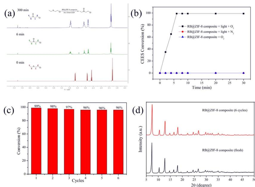
Fig. 5 (a)  $^1\text{H}$  NMR spectrum detection of photooxidation reaction of CEES catalyzed by RB@ZIF-8 composite. (b) Time-dependent conversion of CEES catalyzed by RB@ZIF-8 composite. (c) Recyclability of RB@ZIF-8 composite in the photocatalytic detoxification of CEES. (d) PXRD patterns of the RB@ZIF-8 composite before and after six cycles of CEES degradation.
