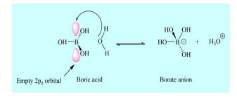
Fig. 1 Structure of boric acid and borate anion. 12
