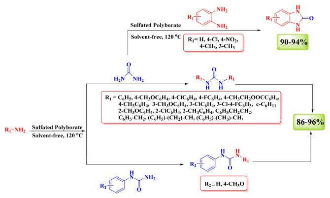
Scheme 18 Synthesis of 1,3-disubstituted urea and 1H-benzimidazol-2(3H)-ones using 10 wt% SPB.
