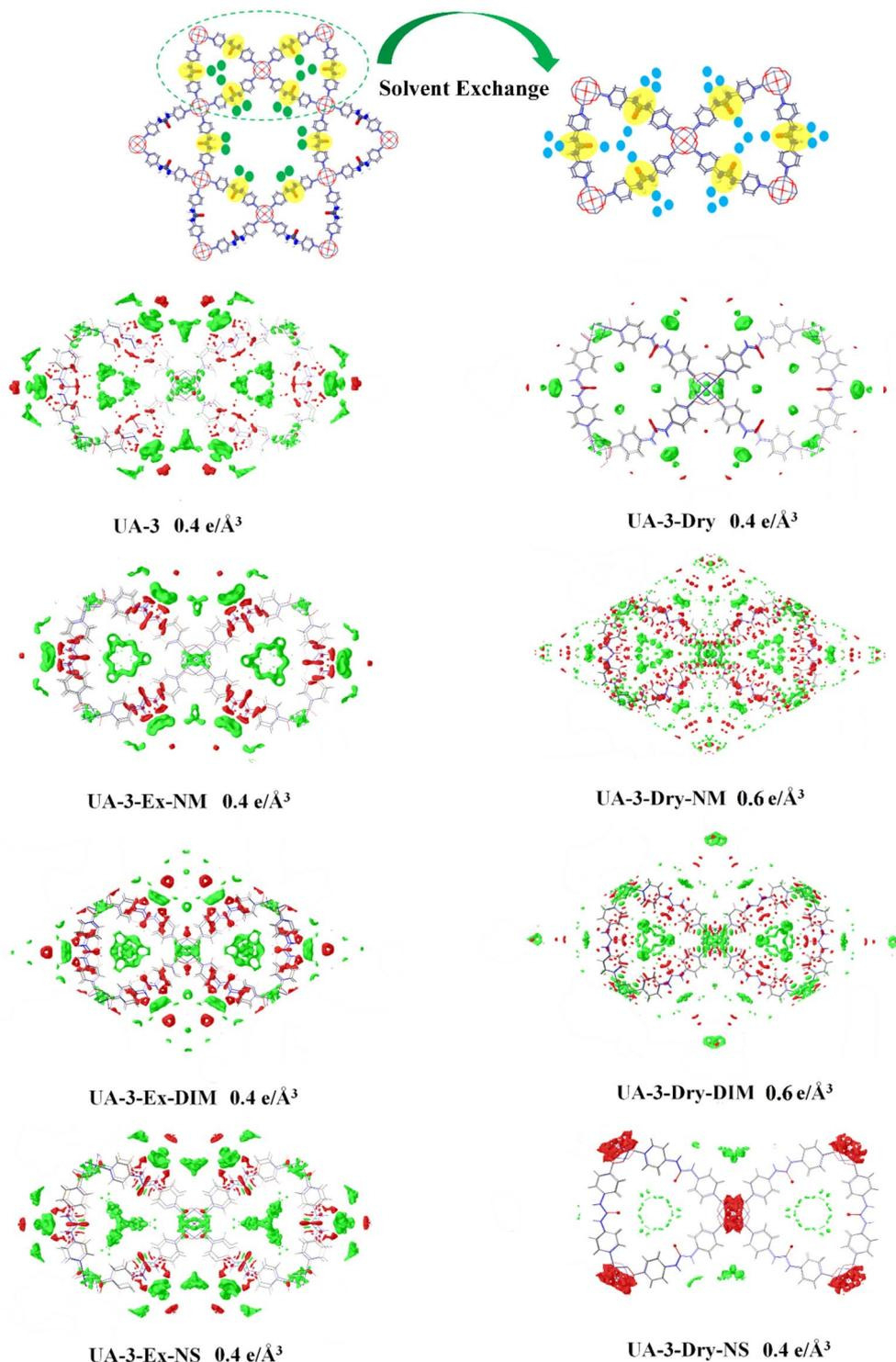
**Fig. 8** Residual electron density maps of the structures without solvent mask: UA-3 native, Dry and UA-3-Ex/Dry.X(guest). The isosurface values of the positive (green) and negative (red) difference electron densities are indicated below the respective figures. For some of the "dry" structures, the isosurface levels have been chosen higher, due to the difference maps being quite noisy due to the inferior data quality yielded by the dried crystals.
