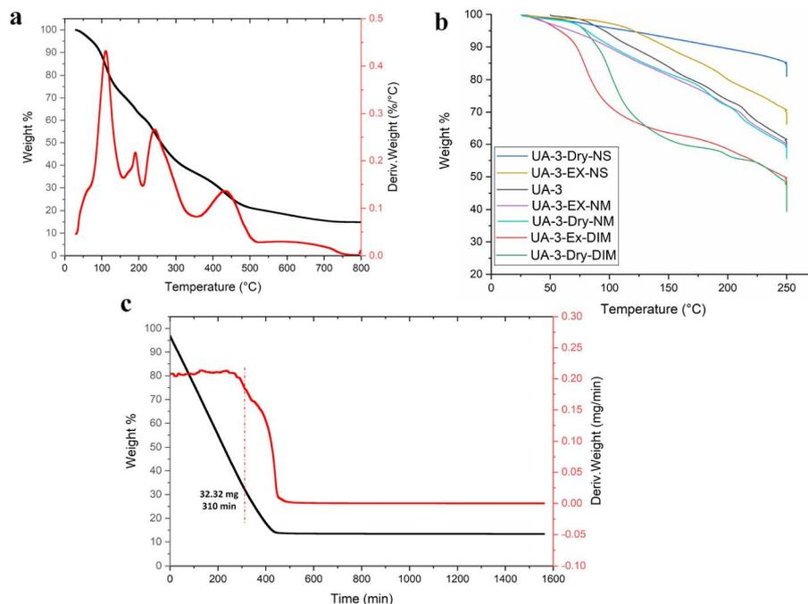
Fig. 9 Thermogravimetric analysis of (a) the as-prepared UA-3 at a heating rate of  $10\text{ }^{\circ}\text{C min}^{-1}$ , showing weight loss and temperature derivative of weight percentage vs. temperature (b) Normalized HR-TGA plots of UA-3 compared with UA-3-Ex-X & UA-3-Dry-X, (c) weight loss profile of UA-3-Dry refilled with DIM under  $\text{N}_2$  at  $23\text{ }^{\circ}\text{C}$ , showing weight loss and the smoothed time derivative of weight percentage vs. time.
