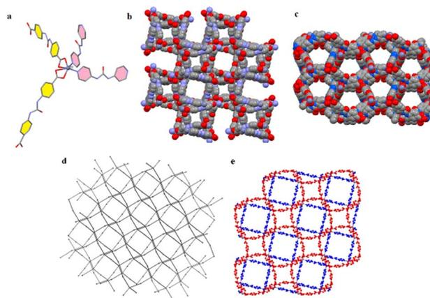
Fig. 3 (a) Representation of the coordination environment around Zn(II) in UA-2, three-dimensional structure along the (b)  $c$  and (c)  $a$  axis (d) simplified view of the polycatenated array with dia; 4/6/c1; sqc6 topology for UA-2, (e) orientation of L1 and L2 linkers within the 3D framework, L1 (red chain) and L2 (blue chain).
