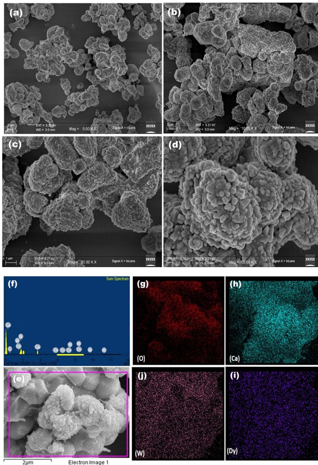
**Fig. 3** (a–d) SEM micrographs of  $\text{Ca}_3\text{WO}_6:1.5 \text{ mol\% Dy}^{3+}$  phosphor at magnifications of 5k $\times$ , 10k $\times$ , 20k $\times$  and 50k $\times$ , respectively. (e) Selected area SEM micrograph, (f) EDAX spectrum and (g–j) elemental mapping of  $\text{Ca}_3\text{WO}_6:1.5 \text{ mol\% Dy}^{3+}$  phosphor for O, Ca, Dy and W, respectively.
