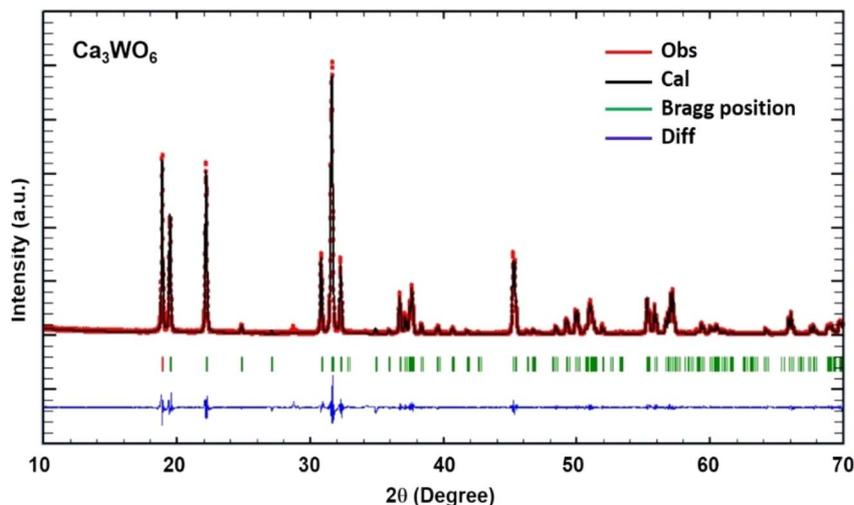
Fig. 1 Rietveld refined the X-ray diffraction profile of undoped  $\text{Ca}_3\text{WO}_6$ .
