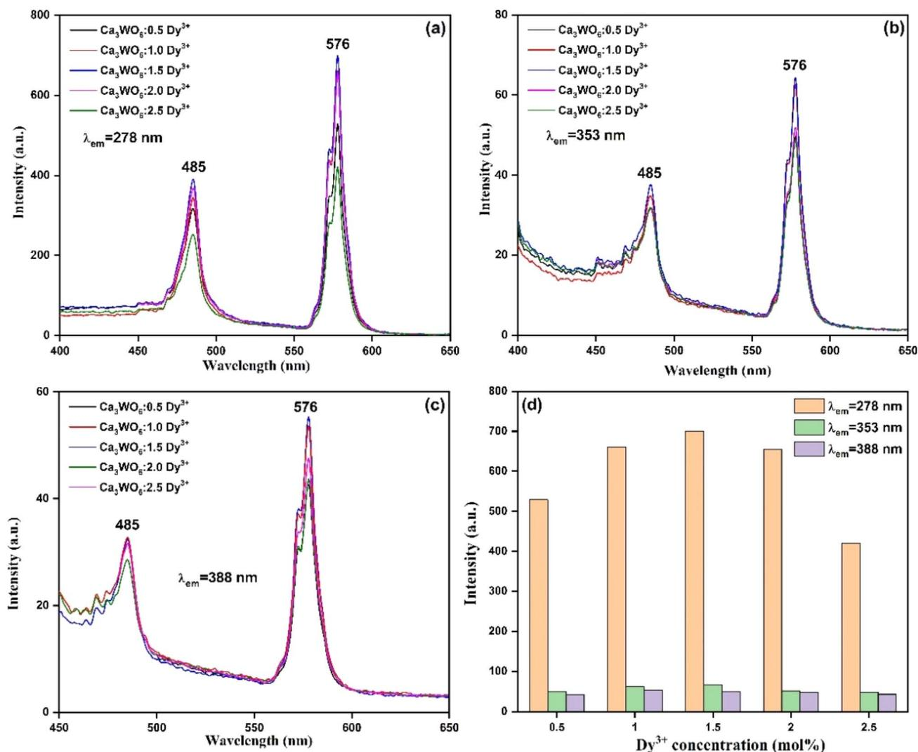
Fig. 6 PL emission spectra of  $Ca_3WO_6:xDy^{3+}$  ( $x = 0.5$ –2.5 mol%) phosphors recorded at (a) 278 nm, (b) 353 nm, and (c) 388 nm; and (d) plot of PL intensity as a function of  $Dy^{3+}$  concentration.
