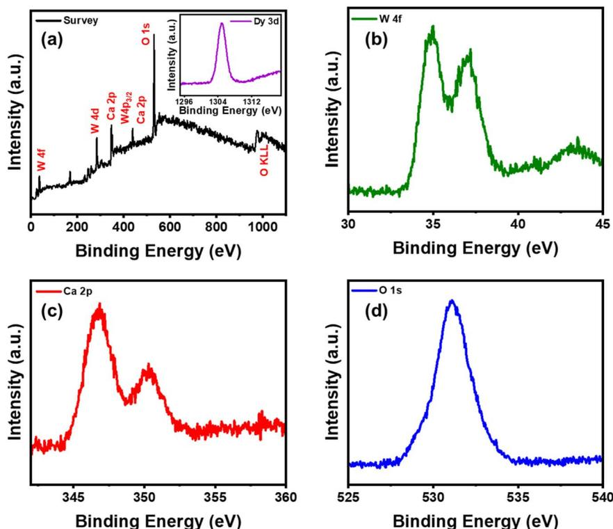
Fig. 4 (a) XPS survey spectra of  $\text{Ca}_3\text{WO}_6:1.5 \text{ mol}\% \text{Dy}^{3+}$  phosphor, inset shows the core-level spectra of Dy, (b–d) shows the core-level spectra of W, Ca and O, respectively.
