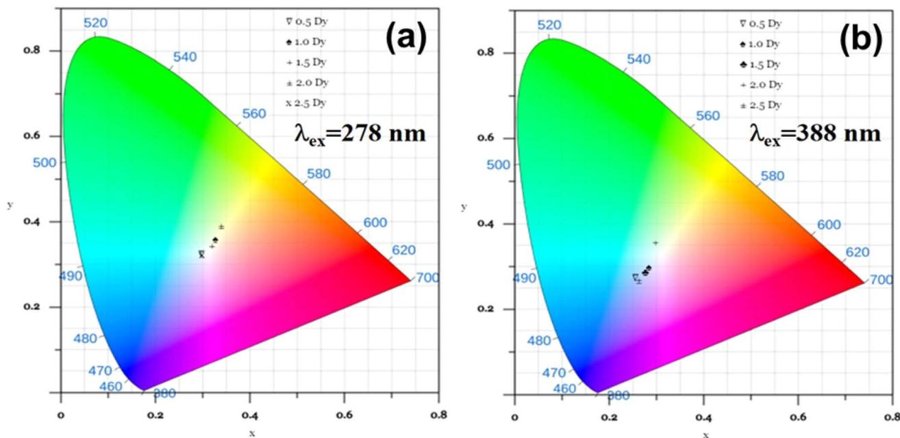
Fig. 10 CIE color coordinates of  $\text{Ca}_3\text{WO}_6:\text{xDy}^{3+}$  ( $\text{x} = 0.5\text{--}2.5$  mol%) phosphors estimated for (a)  $\lambda_{\text{ex}} = 278$  nm and (b)  $\lambda_{\text{ex}} = 388$  nm.
