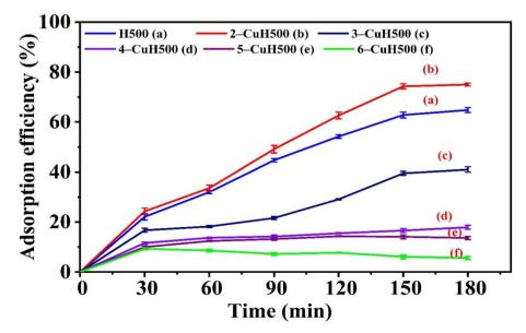
Adsorption efficiency of 100 ppm phenol red (PR) over time on calcined materials H500 and n-CuH500 (n = 2-6).
