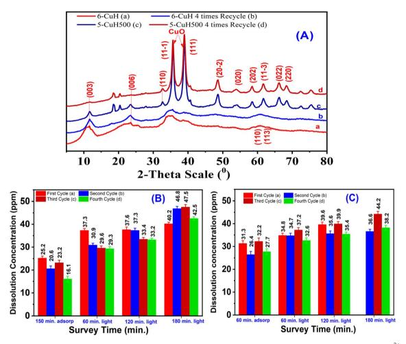
Fig. 23 (A) XRD patterns of 6-CuH and 5-CuH500 materials before and after four reuse cycles; (B) concentration of dissolved  $Cu^{2+}$  ions in the solution from the 6-CuH sample after four reuse cycles; (C) concentration of dissolved  $Cu^{2+}$  ions in the solution from the 5-CuH500 sample after four reuse cycles.
