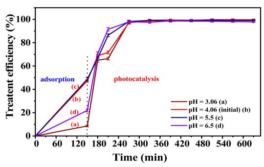
Fig. 19 Time-dependent treatment efficiency of dye compounds in diluted mat-weaving textile wastewater treated with the 5-CuH material in the presence of  $30\% H_2O_2$  under visible light irradiation.
