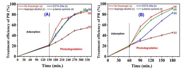
Fig. 17 Degradation efficiency of 100 ppm phenol red (PR) using 6-CuH (A), and 5-CuH500 in the presence and absence of active species and hole scavengers (B).
