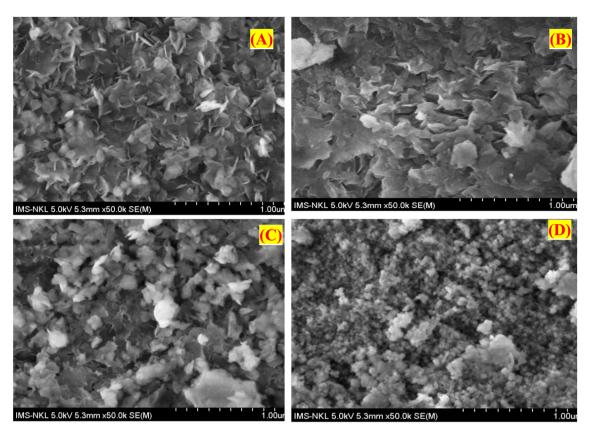
Fig. 4 SEM images of the synthesized material samples (H (A), 5-CuH (B), H500 (C), 5-CuH500 (D)). (H: MgAlCO<sub>3</sub> hydrotalcite, dried at 80 °C for 24 hours; H500: H sample calcined at 500 °C for 5 hours; 5-CuH:  $Cu^{2+}$ -modified hydrotalcite with a  $Cu^{2+}$ /Mg<sup>2+</sup> molar ratio of 5%, dried at 80 °C for 24 hours; 5-CuH500: 5-CuH sample calcined at 500 °C for 5 hours).
