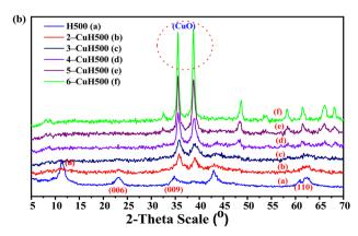
Fig. 1 XRD patterns of the non-calcined (a) and calcined samples (b).
