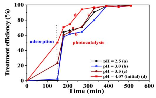
Fig. 20 Time-dependent treatment efficiency of dye compounds in diluted mat-weaving textile wastewater treated with the 5-CuH500 material in the presence of  $30\% H_2O_2$  under visible light irradiation.
