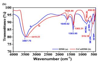
Fig. 3 FT-IR spectra of four material samples: H and 5-CuH (a); H500 and 5-CuH500 (b).
