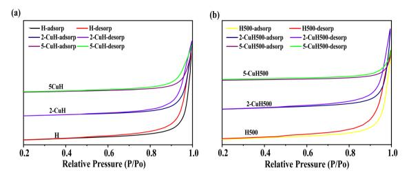
Nitrogen adsorption-desorption isotherms of the synthesized materials of noncalcined materials (a) and calcined materials (b).
