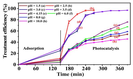
Fig. 16 The treatment efficiency of 100 ppm phenol red over time using 5-CuH500 at different pH values.
