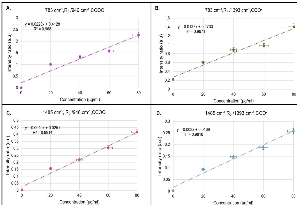
Fig. 4 PLS from peak ratios of lamivudine and AgNPs. (A) 783 cm<sup>-1</sup>/946 cm<sup>-1</sup>; (B) 783 cm<sup>-1</sup>/1393 cm<sup>-1</sup>; (C) 1485 cm<sup>-1</sup>/946 cm<sup>-1</sup>; (D) 1485 cm<sup>-1</sup>/1393 cm<sup>-1</sup>.
