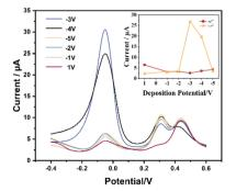
Fig. 10 Effect of enrichment potentials on stripping peaks of Pb<sup>2+</sup> and Cd<sup>2+</sup> in aqueous solutions (vs. Aq/AqCl reference electrode).
