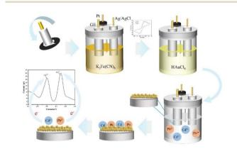
Fig. 1 Detection procedure of Pb<sup>2+</sup> and Cd<sup>2+</sup> via GNPs-Au.
