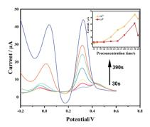
Fig. 11 Optimization of enrichment time for Pb<sup>2+</sup> and Cd<sup>2+</sup> detection via SWASV (vs. Ag/AgCl reference electrode).
