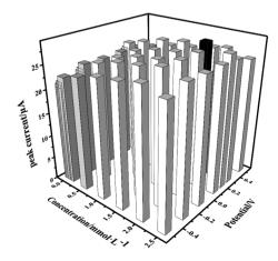
Fig. 3 Dual-parameter optimization of  $\mathsf{HAuCl_4}$  concentrations and deposition potentials.
