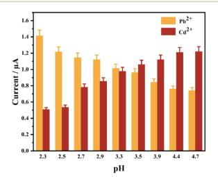
Fig. 8 Variation of  $Pb^{2+}$  and  $Cd^{2+}$  peak currents as different pH (vs. Ag/AgCl reference electrode).
