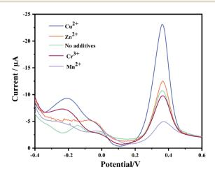
Fig. 14 Interference effects of coexisting heavy metal ions on the stripping peaks of Pb<sup>2+</sup> and Cd<sup>2+</sup> (vs. Ag/AgCl reference electrode).
