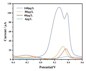
Fig. 15 Stripping peaks of Pb<sup>2+</sup> and Cd<sup>2+</sup> under varying Cu<sup>2+</sup> concentrations (vs. Ag/AgCl reference electrode).
