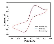
Fig. 2 Cyclic voltammogram of the bare gold electrode (in solution of 0.5 mol per L H<sub>2</sub>SO<sub>4</sub>; vs. Ag/AgCl reference electrode).
