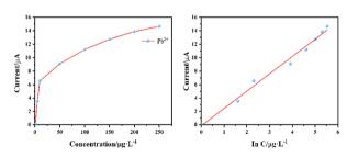
Fig. 12 Linear regression curve of Pb<sup>2+</sup>
