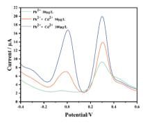
Fig. 9 Stripping voltammogram of Pb<sup>2+</sup> and Cd<sup>2+</sup> at varying concentrations in aqueous solutions (vs. Ag/AgCl reference electrode).
