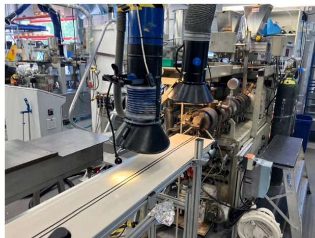
Fig. 1 Production line of monofilaments by Berstorff twin-screw extruder.
