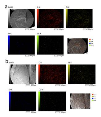
Fig. 6 EDS elemental mapping of CuO NPs dispersed in the cross-section of polyamide 6 monofilaments prepared at a throughput of 3 kg  $h^{-1}$  using: (a) commercial, (b) D CuO NPs.
