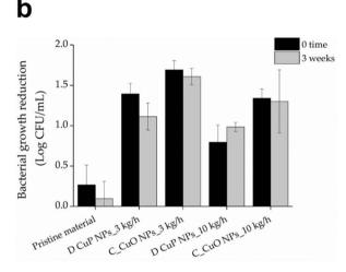
Fig. 10 Antibacterial activity of monofilaments for fish cage net production, composed of 18% BASF PA6, 80% Premix, and 2% D CuO NPs or commercial CuO NPs and produced at 3 or 10 kg h $^{-1}$  extrusion speed, against of the *S. aureus* (a) and *E. coli* (b) at time zero (black bars) and after three-weeks (grey bars) incubation in SMW.
