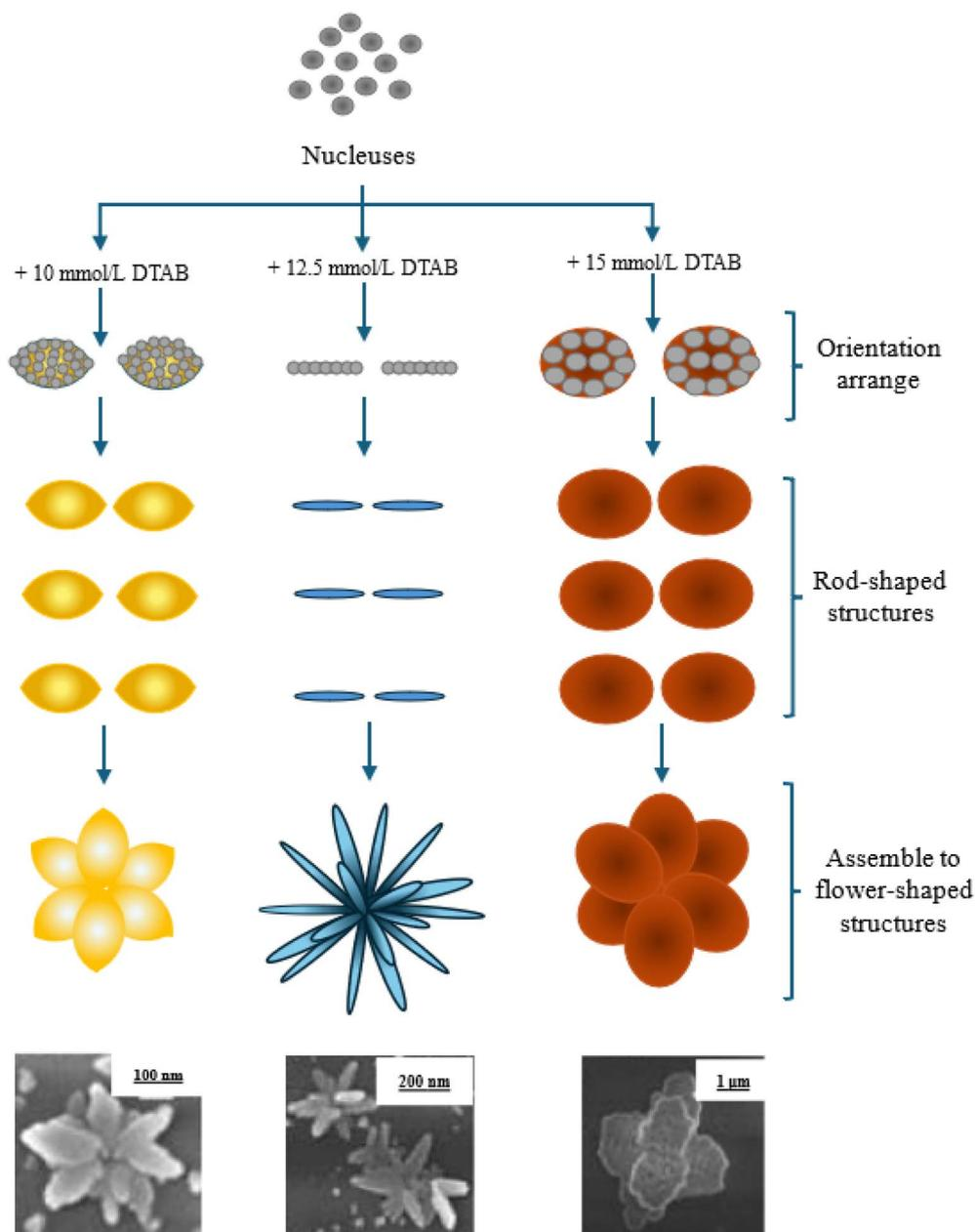
Fig. 8 BaSO<sub>4</sub> nanoparticles growth mechanism with different DTAB concentration.
