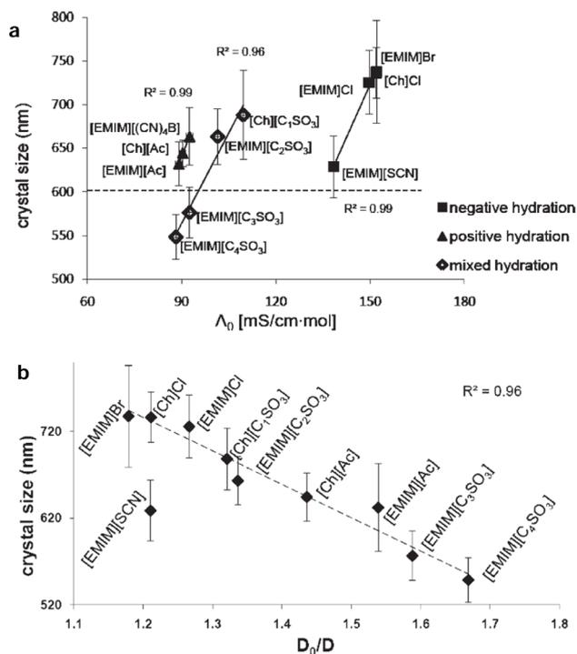
Fig. 9 Correlation curve between BaSO<sub>4</sub> crystal size and (a) limiting molar conductivity ( $\Lambda_0$ ); (b) diffusion in water ( $D_0/D$ ) (reproduced from ref. 125 with permission from the American Chemical Society, copyright 2011).
