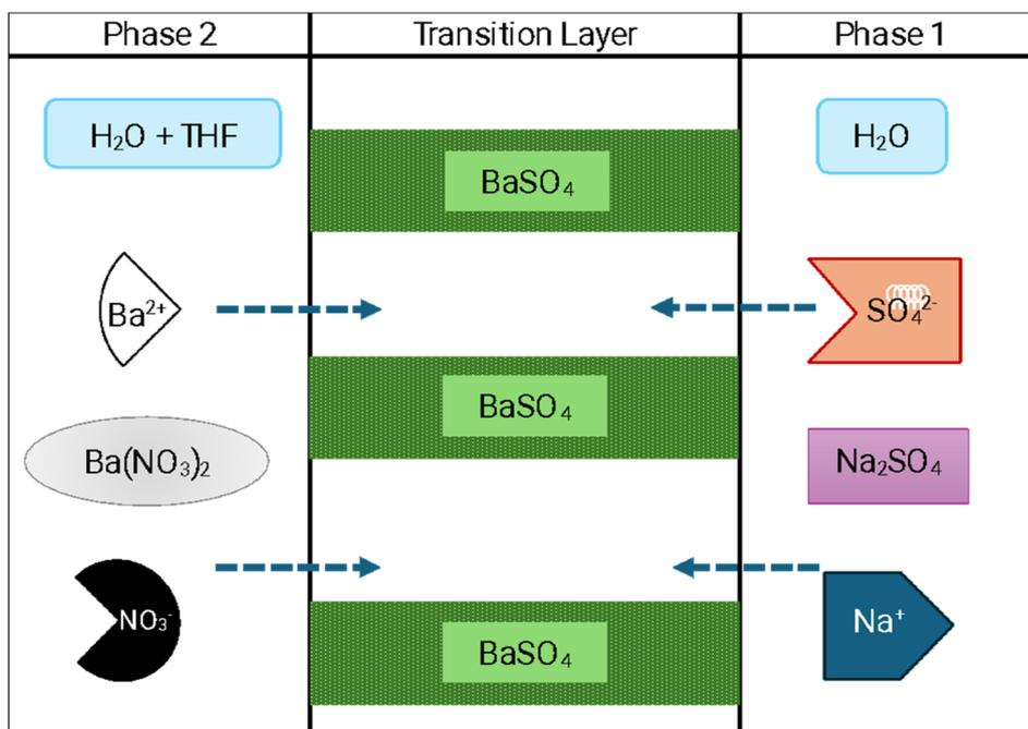
Fig. 4  $\text{BaSO}_4$  nanoparticle precipitation scheme in water–THF system.
