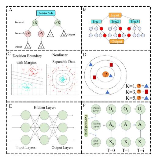
Fig. 2 ML algorithm mechanism diagram. (A) Schematic of DT. (B) Schematic of RF. (C) SVM model diagram including linear and nonlinear models. (D) Schematic of KNN; (E) schematic of an ANN. (F) Schematic of RNN.
