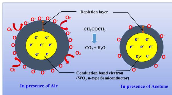
Fig. 10 Schematic representation of acetone gas sensing mechanism.
