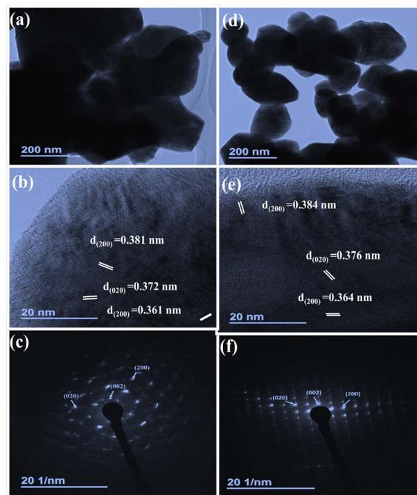
Fig. 6 TEM, HRTEM and SAED analysis of pristine  $\text{WO}_3$  (a–c) and CTAB- $\text{WO}_3$  (d–f), displaying morphological and structural characteristics with indexed SAED patterns.
