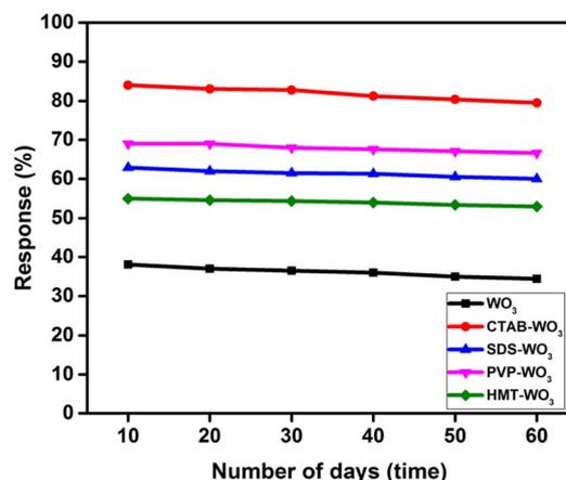
Fig. 13 Long-term stability of sensors response over 60 days.
