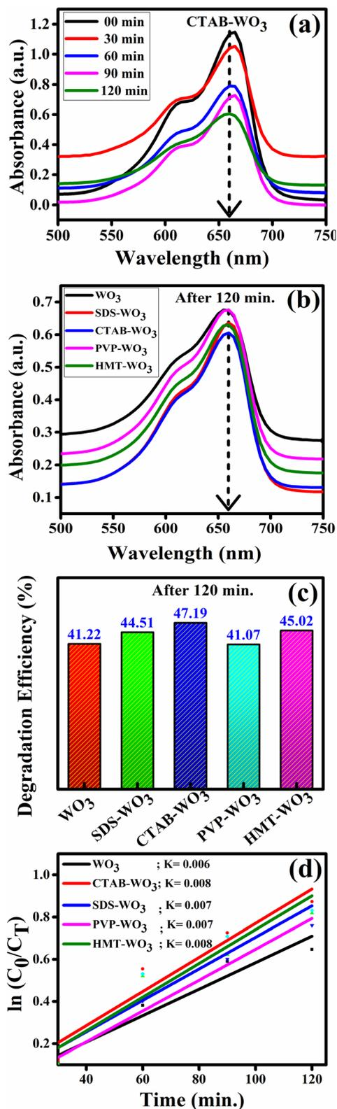
Fig. 14 Photocatalytic activity of surfactant-assisted WO<sub>3</sub>: (a and b) absorbance spectra, (c) degradation efficiency and (d) pseudo-first-order kinetics.
