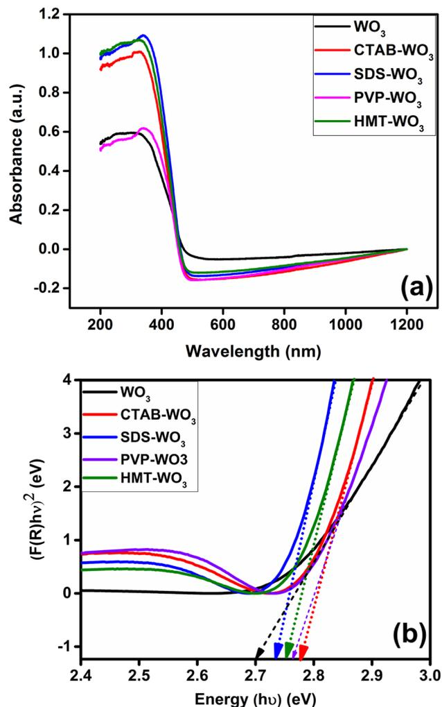
Fig. 8 (a) UV-Vis-NIR absorbance spectra, and (b) Tauc plots of pristine WO<sub>3</sub> and its composites with CTAB, SDS, PVP, and HMT, showing the determination of optical band gap energies ( $E_g$ ).
