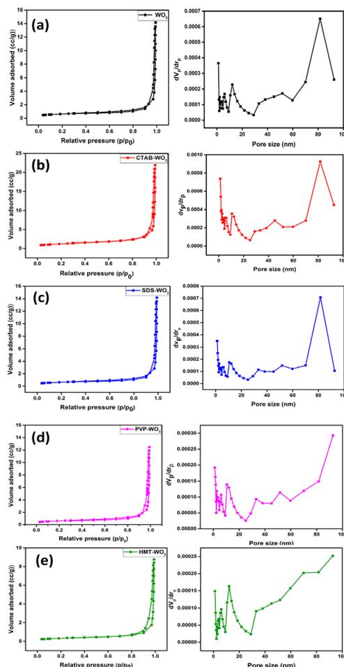
Fig. 9 Nitrogen adsorption–desorption isotherms and pore size distribution of (a) pristine WO<sub>3</sub> (b) CTAB–WO<sub>3</sub> (c) SDS–WO<sub>3</sub> (d) PVP–WO<sub>3</sub> (e) HMT–WO<sub>3</sub>.
