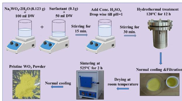
Fig. 2 Synthetic protocols of surfactant assisted- $\text{WO}_3$ .
