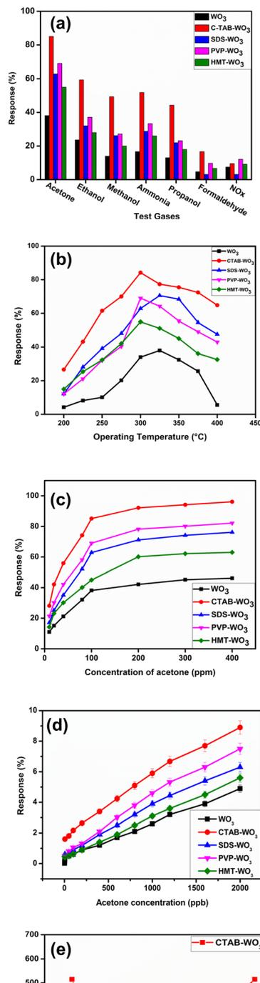
Fig. 11 Gas sensing performance of pristine and surfactant-modified WO<sub>3</sub>: (a) selectivity, (b) operating temperature, (c) acetone concentration variation, (d) acetone sensing performance at ppb level and (e) response/recovery dynamics.
