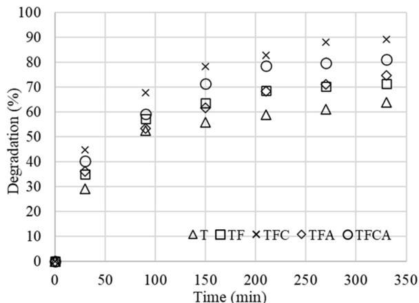
Fig. 4 Effect of photocatalyst (catalyst amount: 0.10 g, pH: 3.0, 0.25 mM  $H_2O_2$ , dye: 50 ppm and UV light exposure: 330 min).
