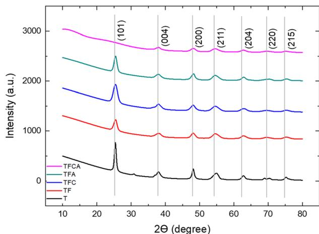
Fig. 2 XRD plot of the prepared nanoparticles.
