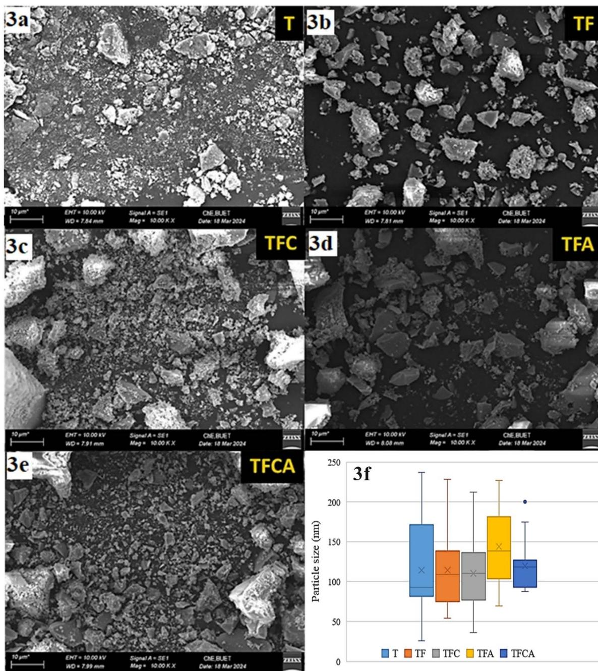
Fig. 3 Microscale SEM images of different nano-photocatalysts; (a) undoped  $\text{TiO}_2$ , (b)  $\text{TiO}_2$  doped with Fe (TF), (c) co-doped with  $\text{Fe}_2\text{O}_3$ - $\text{CeO}_2$  (TFC), (d)  $\text{Fe}_2\text{O}_3$ - $\text{Ag}_2\text{O}$  (TFA), (e)  $\text{Fe}_2\text{O}_3$ - $\text{CeO}_2$ - $\text{Ag}_2\text{O}$  (TFCA) and (f) particle size analysis of different nanophotocatalysts.
