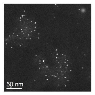
Fig. 4 HAADF-STEM image of the nanoparticle sample after 1 h incubation of a physical Ag/Pt mixture in 3 M KCl. Only particles in the  $\sim$ 3 nm size range were observed; the  $\sim$ 10 nm silver nanoparticles that had been present in the original dispersion were no longer detectable.
