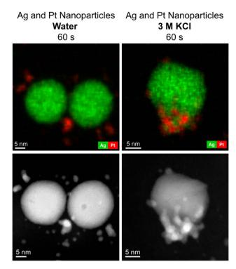
Fig. 3 Energy-dispersive X-ray maps (top) and corresponding HAADF-STEM micrographs of silver and platinum nanoparticles (bottom) after immersion in water (left) or 3 M KCl solution (right) for 60 s.
