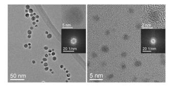
Fig. 1 Transmission electron micrographs and corresponding FFT insets of silver (left) and platinum (right) nanoparticles.
