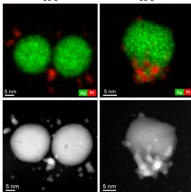
**Fig. 3** Energy-dispersive X-ray maps (top) and corresponding HAADF-STEM micrographs of silver and platinum nanoparticles (bottom) after immersion in water (left) or 3 M KCl solution (right) for 60 s.
