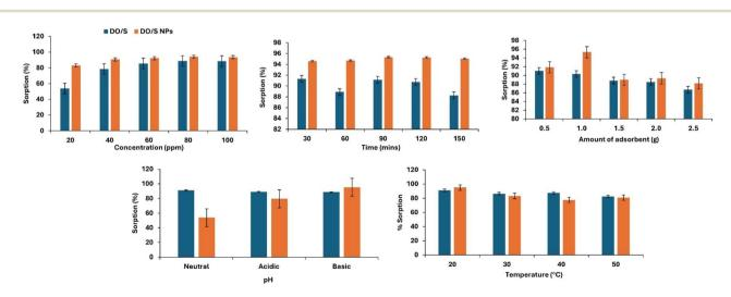
Fig. 11 A comparison of the impacts of concentration, time, adsorbent dose, pH, and temperature on crystal violet adsorption.
