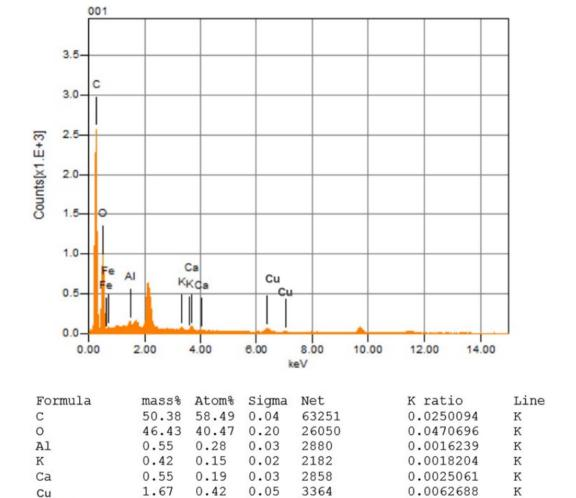
Fig. 7 EDX results of DO/S NPs.
