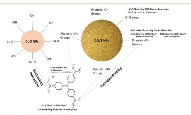
Fig. 15 Adsorption mechanism of DO/S and DO/S NPs
