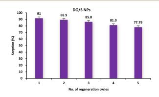
Fig. 16 Regeneration of DO/S NPs for dye removal.
