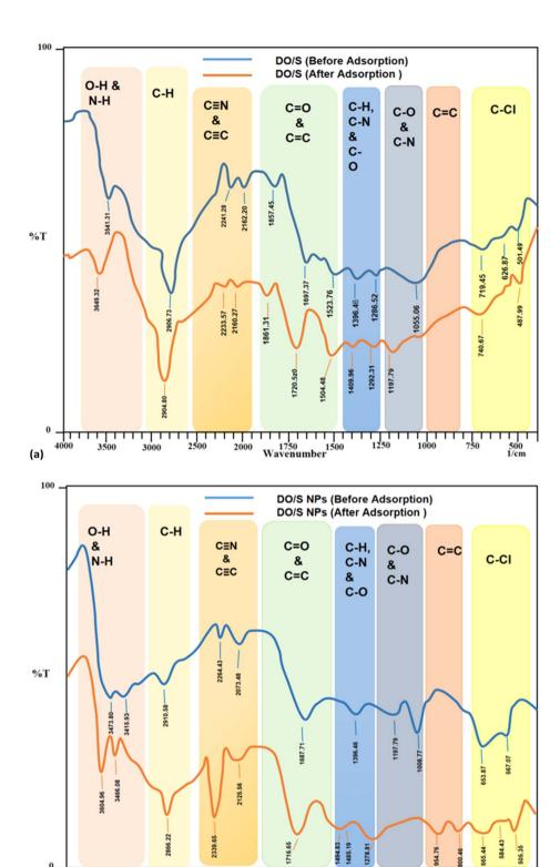
Fig. 3 (a) FTIR spectra of de-oiled Glycine max L. (before and after adsorption). (b) FTIR spectra of de-oiled Glycine max L. loaded with Cu NPs (before and after adsorption).
