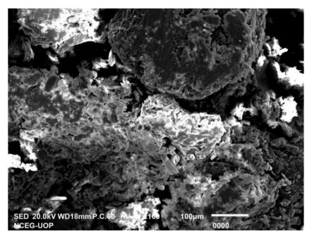
Fig. 4 SEM of DO/S NPs at 100  $\mu m$  and  $\times 160$  magnification.
