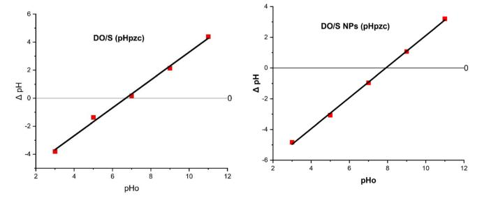
Fig. 8 pH PZC determination of DO/S and DO/S NPs.
