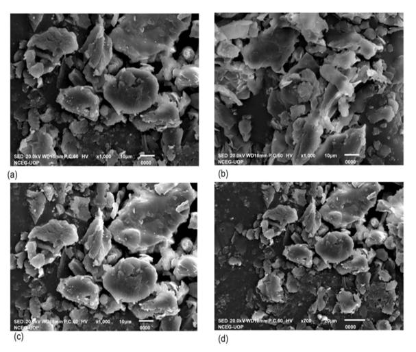
Fig. 6 SEM Of DO/S NPs at different scale bars and magnifications: (a)  $10 \mu m$ ,  $\times 1000$ ; (b)  $10 \mu m$ ,  $\times 1000$ ; (c)  $10 \mu m$ ,  $\times 1000$ ; and (d)  $20 \mu m$ ,  $\times 700$ .
