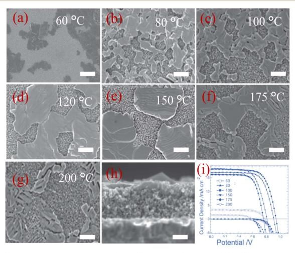
Fig. 4 (a-g) SEM of perovskite films deposited onto m-TiO<sub>2</sub> films, (h) cross sectional SEM image at 150 °C, and (i) J-V curves of the assembled FPSC devices. Reprinted with permission from ref. 107 Copyright 2014, Wiley-VCH.
