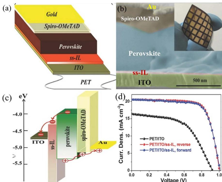
Fig. 10 (a) Device structure, (b) cross-sectional SEM of FPSC with ss-IL as ETL, (c) energy-level, and (d)  $J$ - $V$  curve of the best device. Reprinted with permission from ref. 144. Copyright 2016, Wiley-VCH.
