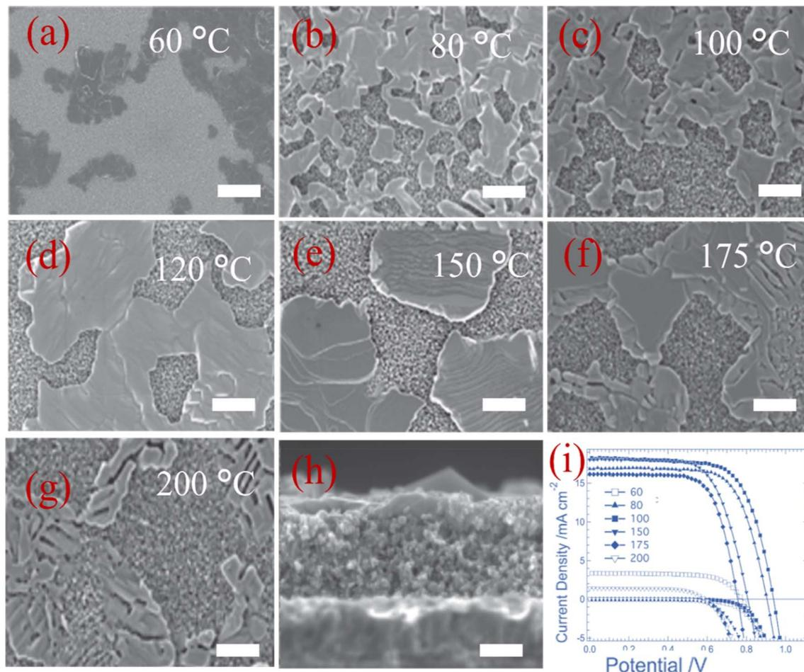
Fig. 4 (a–g) SEM of perovskite films deposited onto  $m\text{-TiO}_2$  films, (h) cross sectional SEM image at 150 °C, and (i)  $J$ – $V$  curves of the assembled FPSC devices. Reprinted with permission from ref. 107 Copyright 2014, Wiley-VCH.
