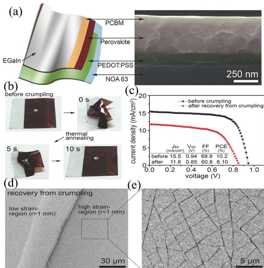
Fig. 15 (a) Scheme of the stacked layers on an NOA63 film and a cross-sectional SEM image of the device, (b) photographs of the device during the crumpling test, (c)  $J$ - $V$  curves before crumpling and after shape recovery from crumpling test, (d) SEM and (e) magnified SEM images of the top surface after shape recovery from crumpling test showing regions of low strain and high strain. Reprinted with permission from ref. 90. Copyright 2015, Wiley-VCH.
