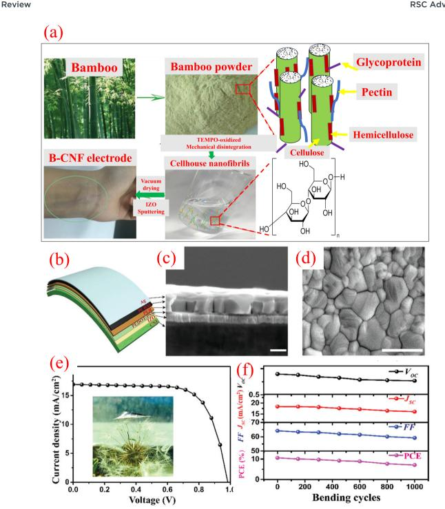
Fig. 22 (a) Scheme of the preparation of b-CNF electrodes, (b) scheme of the FPSCs, (c) cross-section SEM image of the perovskite films based on the b-CNF electrode, (d) top-view SEM image of the perovskite film, (e) J-V curve of the b-CNF-based FPSCs, and (f) main parameter variation of the FPSCs upon bending tests at a 4 mm radius. Reprinted with permission from ref. 196. Copyright 2019, Wiley-VCH.
