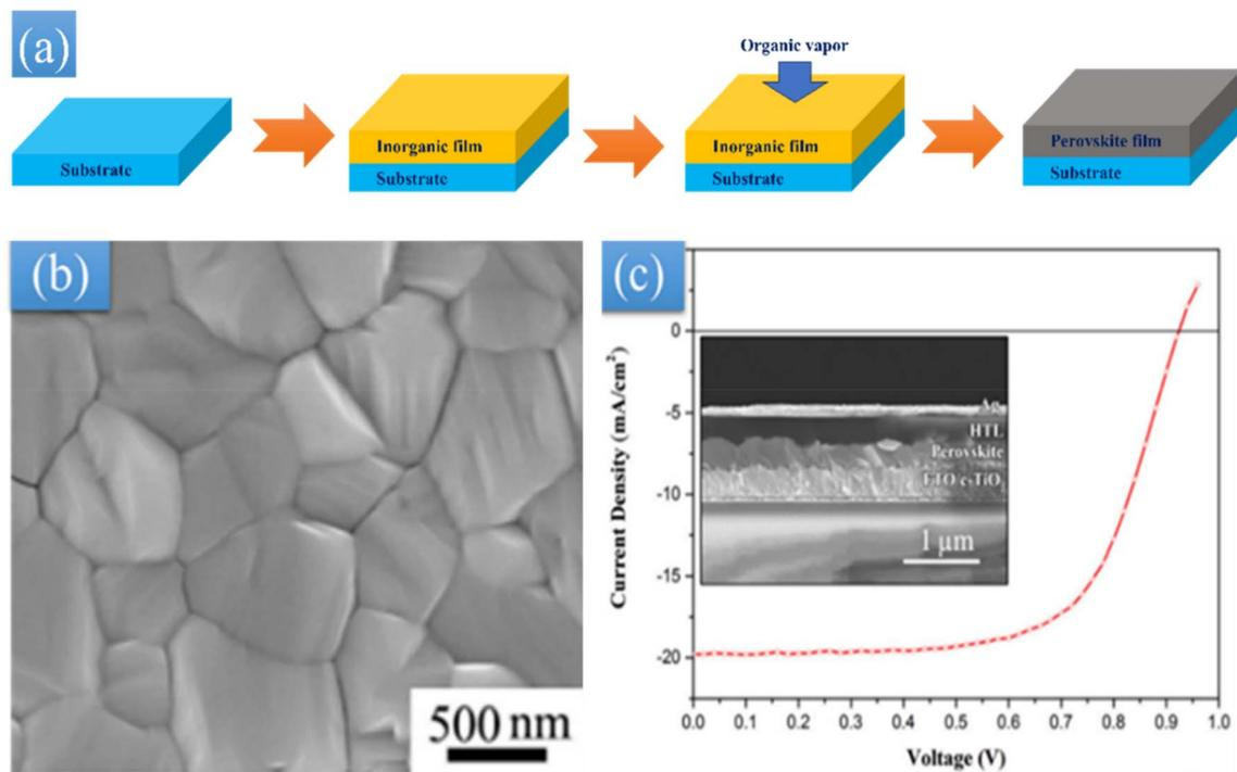
Fig. 8 (a) Scheme for the formation of the perovskite film through the vapour-assisted solution method, (b) SEM image of the perovskite film at 150 °C for 4 h, and (c)  $J$ - $V$  curve of PSCs based on the as-prepared perovskite films (inset is the cross-sectional SEM of the FPSC). Reprinted with permission from ref. 132. Copyright 2014, American Chemical Society.
