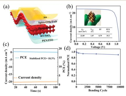
Fig. 13 (a) Scheme of the FPSC device, (b) J-V curve, (c) stabilized current density and PCE, and (d) normalized PCE as a function of bending cycles at a radius of 5 mm. Reprinted with permission from ref. 155. Copyright 2022, Wiley-VCH.
