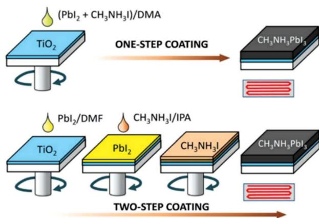
Fig. 5 Fabrication of  $\text{CH}_3\text{NH}_3\text{PbI}_3$  films via one-step and two-step spin-coating techniques. Reprinted with permission from ref. 117 Copyright 2014, AIP Publishing.
