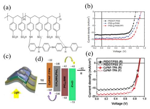
Fig. 16 (a) Chemical structure of PSS-g-PANI and (b) J-V curves of the devices with PEDOT:PSS, PSS-g-PANI, and PSS-g-PANI: PFI HTLs. Reprinted with permission from ref. 172. Copyright 2016, Wiley-VCH. (c) Flexible structure, (d) energy level, and (e) J-V curves of the FPSC with PEDOT:PSS. Reprinted with permission from ref. 173. Copyright 2017, Elsevier.
