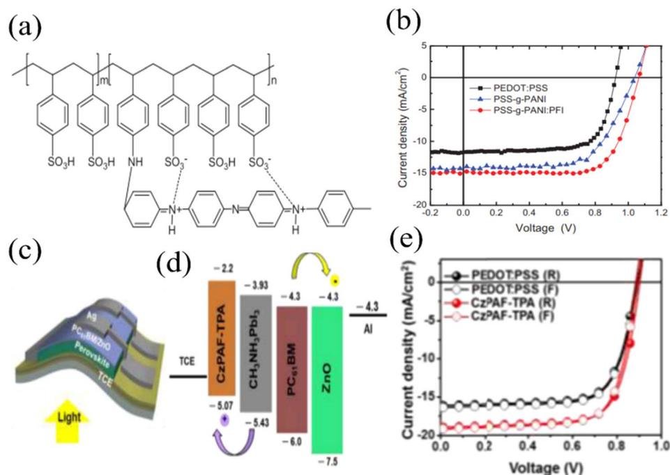
Fig. 16 (a) Chemical structure of PSS-g-PANI and (b)  $J$ - $V$  curves of the devices with PEDOT:PSS, PSS-g-PANI, and PSS-g-PANI:PFI HTLs. Reprinted with permission from ref. 172. Copyright 2016, Wiley-VCH. (c) Flexible structure, (d) energy level, and (e)  $J$ - $V$  curves of the FPSC with PEDOT:PSS. Reprinted with permission from ref. 173. Copyright 2017, Elsevier.
