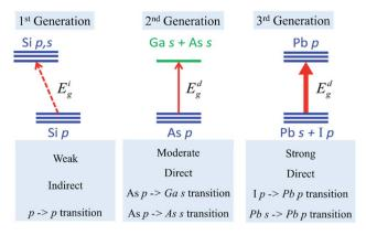
Fig. 1 Scheme representing the optical absorption of the absorbers in the 1st, 2nd, and 3rd generations of PVs. Reprinted with permission from ref. 49. Copyright 2015, Royal Society of Chemistry.
