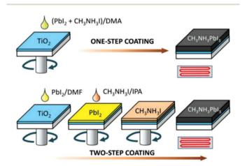
Fig. 5 Fabrication of  $CH_3NH_3PbI_3$  films  $\emph{via}$  one-step and two-step spin-coating techniques. Reprinted with permission from ref. 117 Copyright 2014, AIP Publishing.
