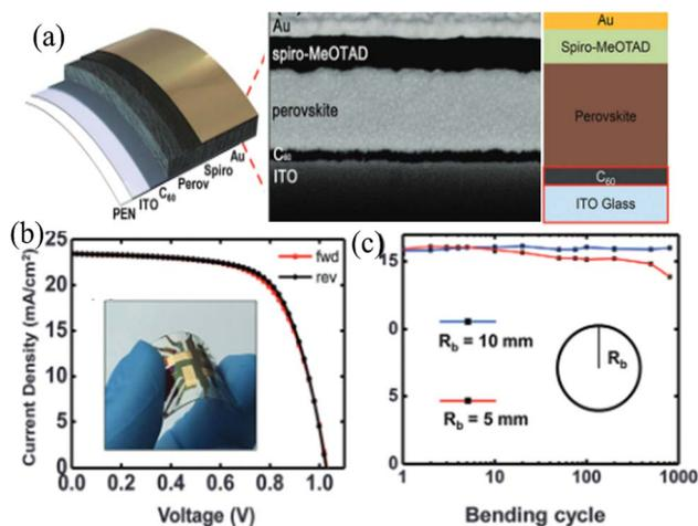
Fig. 14 (a) Scheme of the FPSC with a cross-sectional SEM image, (b)  $J$ - $V$  curve, and (c) efficiency as a function of bending cycles with radii of 10 mm and 5 mm. Reprinted with permission from ref. 160. Copyright 2016, Royal Society of Chemistry.
