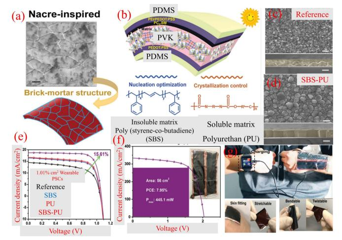
Fig. 26 (a) Brick-mortar structure, (b) structure of wearable FPSCs with chemical structures of SBS and PU. Top-view and cross-section SEM images of (c) reference and (d) SBS-PU-based films. (e) J-V curves of the related devices, (f) I-V curves of a wearable solar-power source with SBS-PU (inset is the photograph of assembled device), and (g) photographs of wearable FPSCs as a power source to power a smartwatch. Reprinted with permission from ref. 214. Copyright 2019, Royal Society of Chemistry.
