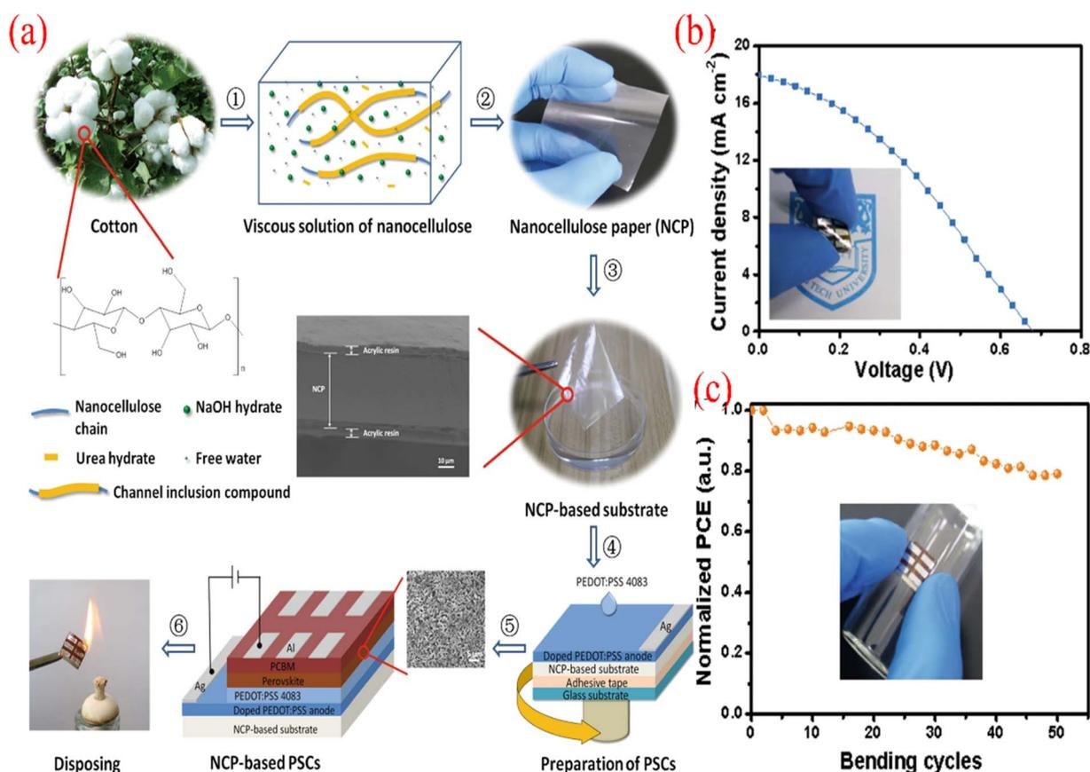
Fig. 21 (a) Scheme of the process of NCP-based substrate and NCP-FPSC, (b)  $J$ - $V$  curves of NCP-FPSC, and (c) normalized PCE-bending cycles state on a bottle with a diameter of 15 mm. Reprinted with permission from ref. 195. Copyright 2019, Springer Nature.
