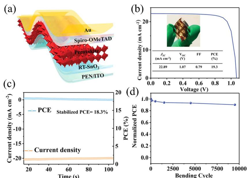
Fig. 13 (a) Scheme of the FPSC device, (b)  $J$ - $V$  curve, (c) stabilized current density and PCE, and (d) normalized PCE as a function of bending cycles at a radius of 5 mm. Reprinted with permission from ref. 155. Copyright 2022, Wiley-VCH.
