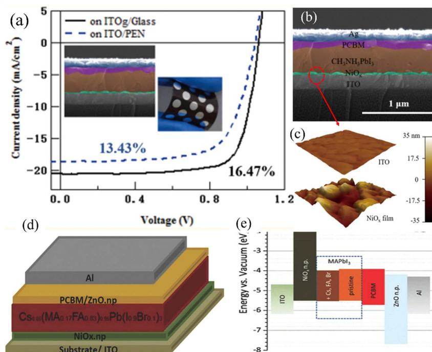
Fig. 18 (a) *J*–*V* curves of the devices based on NiO<sub>x</sub> layers, (b) cross-sectional SEM image of the NiO<sub>x</sub>-based FPSC, and (c) AFM images of ITO and the NiO<sub>x</sub> film on the ITO substrate. Reprinted with permission from ref. 177. Copyright 2016, American Chemical Society. (d) Architecture of the inverted planar PSCs and (e) energy levels of the layers. Reprinted with permission from ref. 182 Copyright 2018, Wiley-VCH.
