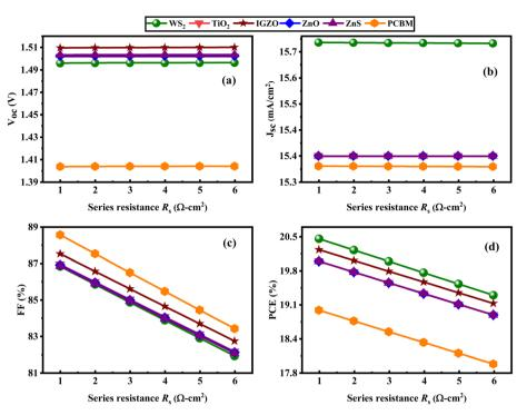
Fig. 12 Series resistance  $R_s$  affects the following performance metrics: (a)  $V_{OC}$ , (b)  $J_{SC}$ , (c) FF, (d) PCE of (ITO/ETL/LiMgI<sub>3</sub>/Cu<sub>2</sub>O/Ni) ETL = WS<sub>2</sub>, TiO<sub>2</sub>, IGZO, ZnO, ZnS, and PCBM.
