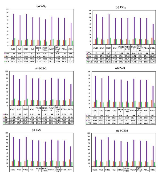
Fig. 6 The change in performance parameters such as  $V_{\rm OC}$  (V),  $J_{\rm SC}$  (mA cm<sup>-2</sup>), FF (%), PCE (%) is studied for LiMgI<sub>3</sub> absorber-based PSCs with various HTLs and Ni as the back metal contact, using ETLs of (a) WS2, (b) TiO2, (c) IGZO, (d) ZnO, (e) ZnS, and (f) PCBM.
