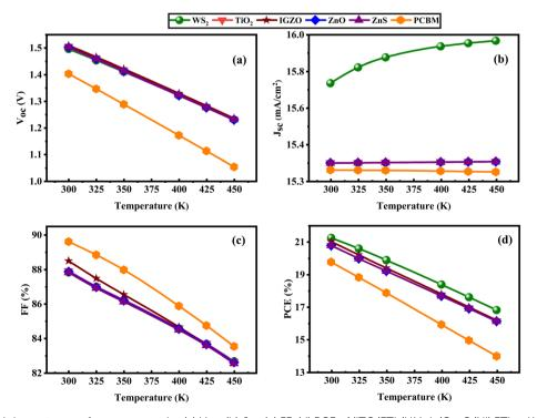
Fig. 14 Temperature's impact on performance metrics (a)  $V_{OC}$ , (b)  $J_{SC}$ , (c) FF, (d) PCE of (ITO/ETL/LiMgI<sub>3</sub>/Cu<sub>2</sub>O/Ni) ETL = WS<sub>2</sub>, TiO<sub>2</sub>, IGZO, ZnO, ZnS, and PCBM.
