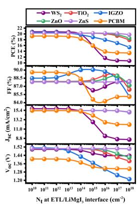
Fig. 17 Investigating the influence of ETL/LiMgl<sub>3</sub> interface defect levels on  $V_{\rm OC}$  (V),  $J_{\rm SC}$  (mA cm<sup>-2</sup>), FF (%), and PCE (%) of LiMgl<sub>3</sub>.
