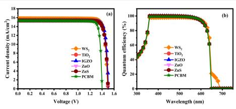
Fig. 16 (a) J-V characteristics and (b) QE response of the single halide PSCs.
