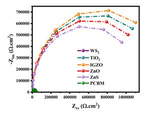
Fig. 18 Nyquist plot of the various ETL materials (WS<sub>2</sub>, TiO<sub>2</sub>, IGZO, ZnO, ZnS, and PCBM) based structure with LiMgl<sub>3</sub> absorber.
