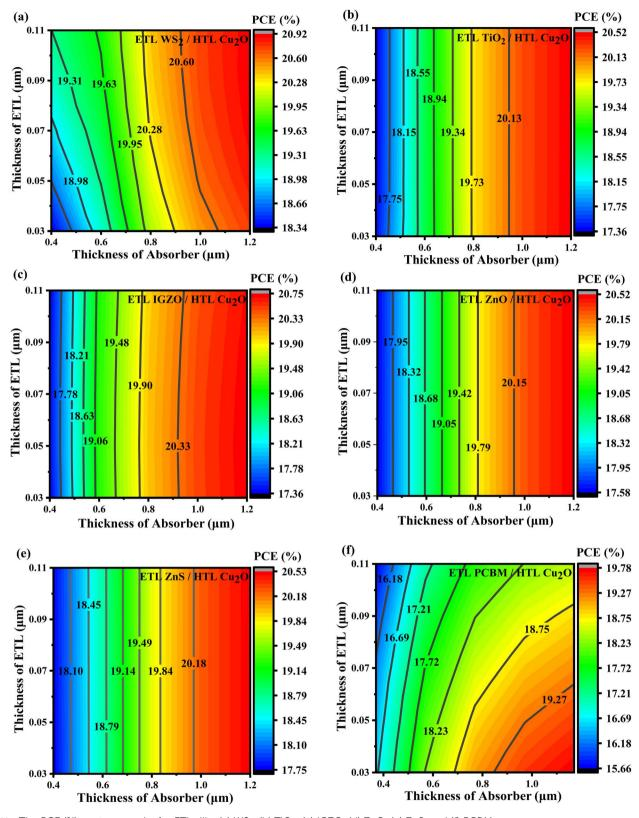
Fig. 11 The PCE (%) contour graphs for ETLs like (a)  $WS_2$ , (b)  $TiO_2$ , (c) IGZO, (d) ZnO, (e) ZnS, and (f) PCBM.
