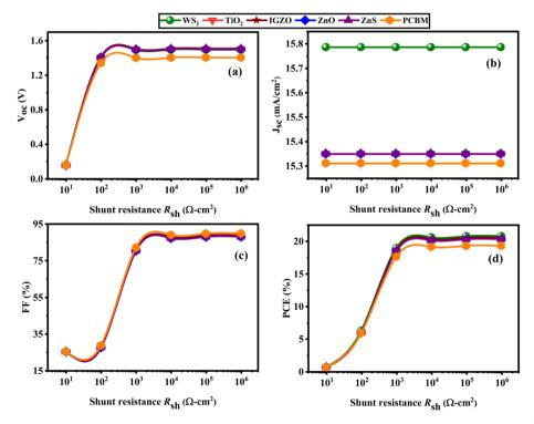
Fig. 13 Shunt resistance  $R_{\rm sh}$  affects the following performance metrics: (a)  $V_{\rm OC}$ , (b)  $J_{\rm SC}$ , (c) FF, (d) PCE of (ITO/ETL/LiMgI<sub>3</sub>/Cu<sub>2</sub>O/Ni) ETL = WS<sub>2</sub>, TiO<sub>2</sub>, IGZO, ZnO, ZnS, and PCBM.
