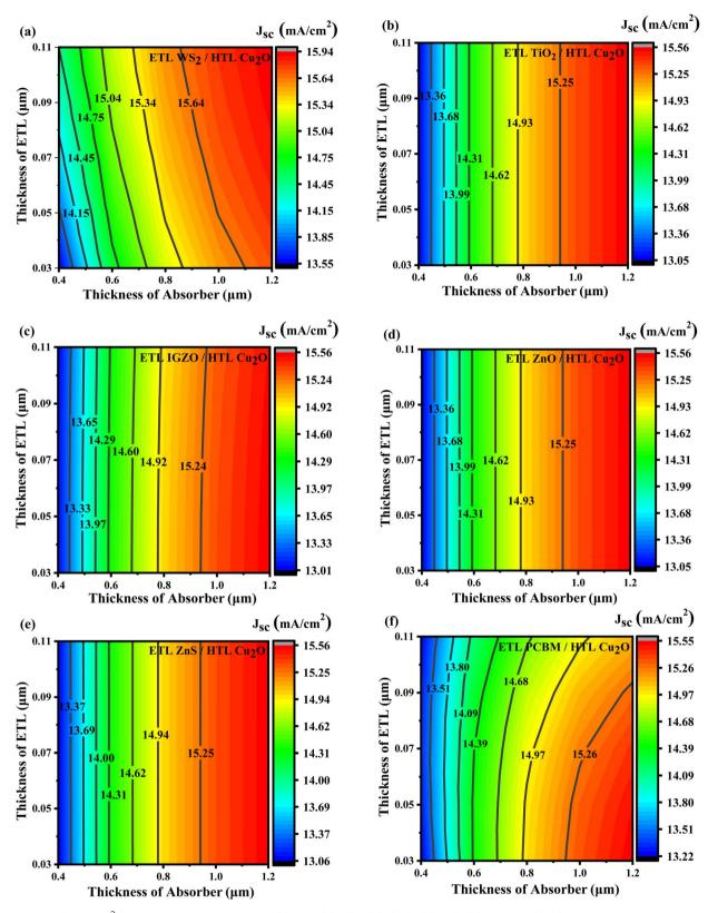
Fig. 9 The  $J_{SC}$  (mA cm<sup>-2</sup>) contour graphs for ETLs like (a) WS<sub>2</sub>, (b) TiO<sub>2</sub>, (c) IGZO, (d) ZnO, (e) ZnS, and (f) PCBM.
