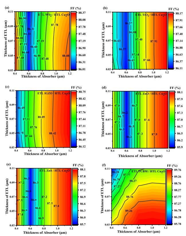
Fig. 10 The FF (%) contour graphs for ETLs like (a) WS2, (b) TiO2, (c) IGZO, (d) ZnO, (e) ZnS, and (f) PCBM.
