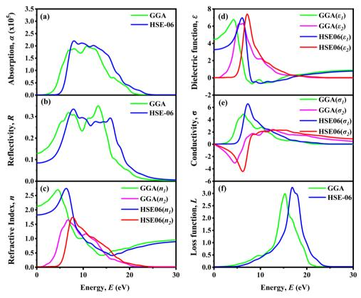
Fig. 5 Optical properties: (a) absorption, (b) reflectivity, (c) refractive index, (d) dielectric function, (e) conductivity and (f) loss function for LiMql<sub>3</sub>.
