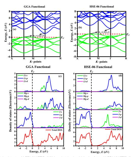
Fig. 4 Electronic band structure (a) GGA, (b) HSE06 of LiMgl<sub>3</sub>, and total and partial density of states (c) GGA, (d) HSE06 of LiMgl<sub>3</sub>.
