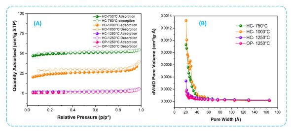
Fig. 5 (A) N<sub>2</sub> adsorption-desorption isothermal curves, and (B) pore size distribution of HC for different temperatures
