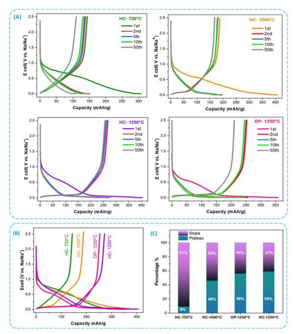
Fig. 7 (A) Galvanostatic charge/discharge curves of HC electrodes at 25 mA  $\rm g^{-1}$ , (B) comparison of charge/discharge profiles of HC during the first cycle, and their (C) sloping and plateau capacity of each electrode at different temperatures.
