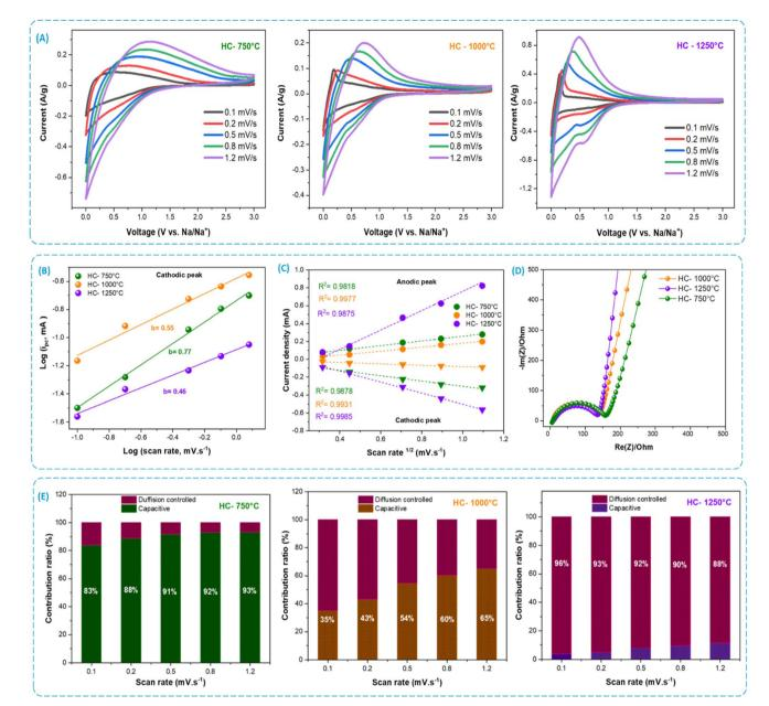
Fig. 9 (A) CV curves at various scan rates from 0.1 to 1.2 mV s<sup>-1</sup>, (B) linear relationship between  $\log(i)$  vs.  $\log(v)$  for the samples, (C) linear relation between peak current ip and the square root of various scan rate  $v^{1/2}$ , (D) impedance spectroscopy of the samples, (E) the capacity contribution at various scan rates
