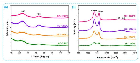
Fig. 4 (A) XRD and (B) Raman spectrums of HC samples for different temperatures.
