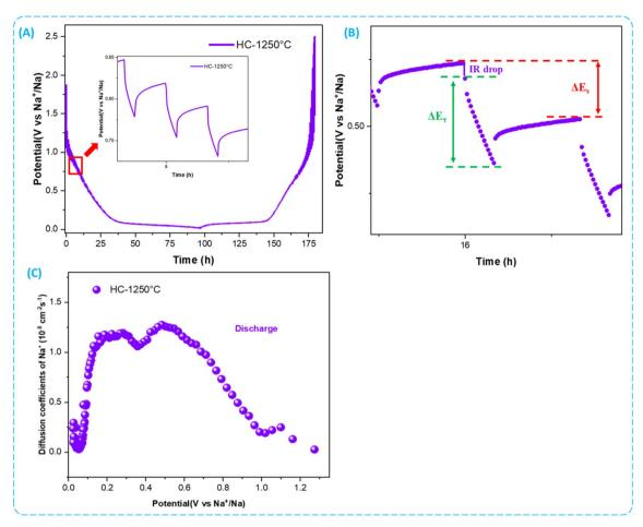
Fig. 10 (A) The GITT curves of HC-1250 °C, (B) potential profile of constant current pulse with schematic labeling of different parameters, (C)  $D_{\text{Na}^+}$  diffusion coefficients calculated from the GITT for discharge process.
