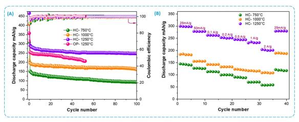
Fig. 8 Electrochemical performance of the HC electrodes at different temperatures (A) capacity retention and the coulombic efficiency, (B) rate performance at different current densities.
