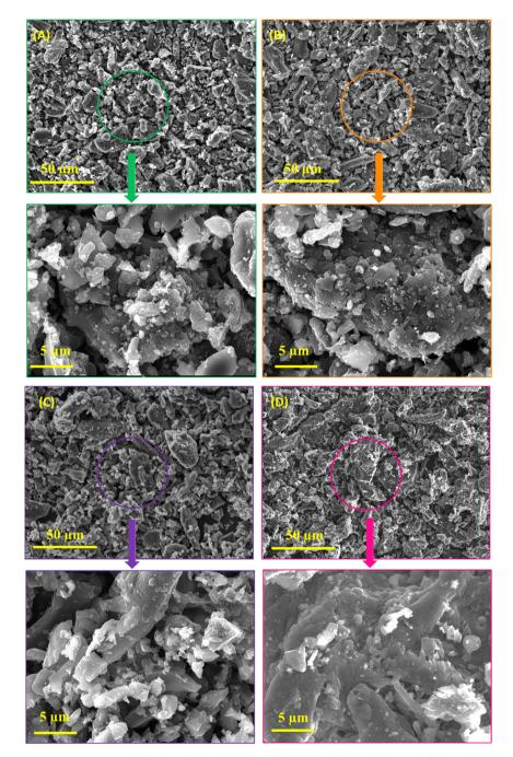
Fig. 2 SEM images and their magnifications of (A) HC-750 °C, (B) HC-1000 °C, (C) HC-1250 °C, and (D) OP-1250 °C.
