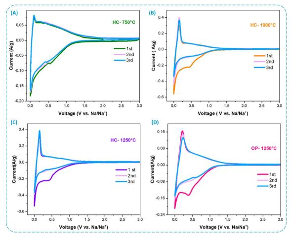
Fig. 6 CV curves at a scan rate of 0.1 mV s $^{-1}$  of (A) HC-750, (B) HC-1000, (C) HC-1250, and (D) OP-1250 °C.
