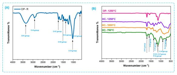
Fig. 1 (A) FT-IR spectra of OP-R, (B) of HCs obtained for different temperatures.
