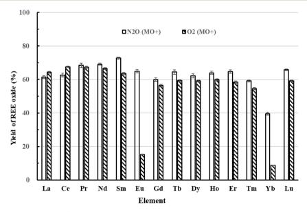
Fig. 1 Yields of REE oxides using the ICP-MS/MS mass-shift method with  $O_2$  or  $N_2O$  as the cell gas. The flow rate of  $O_2$  or  $N_2O$  was 1.2 mL min<sup>-1</sup>, and the concentration of REE was 1  $\mu$ g L<sup>-1</sup>.
