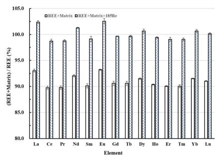
Fig. 2 Comparison of the matrix effects between REE<sup>+</sup> signals caused by a matrix with or without  $^{185}$ Re as the internal standard. The matrix comprised 10, 5, 5, and 1 mg L<sup>-1</sup> Na, Ca, Mg and K, respectively, and the concentration of REEs was 0.2  $\mu$ g L<sup>-1</sup>.
