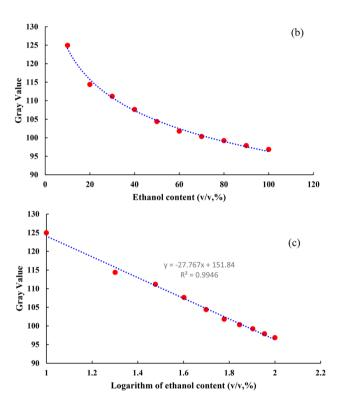
Fig. 4 Profile plots of the plate showing the variation in gray value with pixel (a), variation in gray value in minima with ethanol content (b) and variation in gray value with logarithm of ethanol content (c). Values on the curve (a) indicate the ethanol contents of the mixtures.
