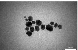
Fig. 1 TEM micrographs of the AgNPs synthesized in the presence of citrate using walnut peel extract.
