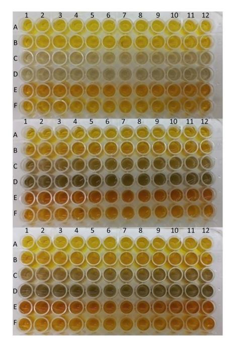
Fig. 3 Image of three replicates of the constructed sensor array. Each row in the array corresponds to AgNPrs reported in Table 2 and each column corresponds to the mixtures reported in Table 1.
