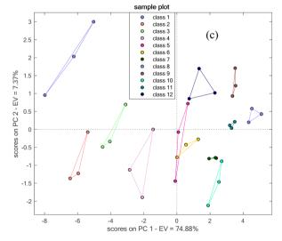
Fig. 5 Score plots obtained by analysis of the RGB data from the image of the sensor array (Fig. 3) via PCA without preprocessing (a), after mean centering (b) and after auto-scaling (c).
