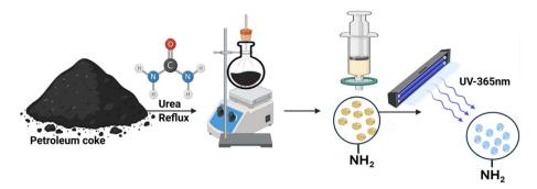
Scheme 1 Schematic illustration of the preparation steps.
