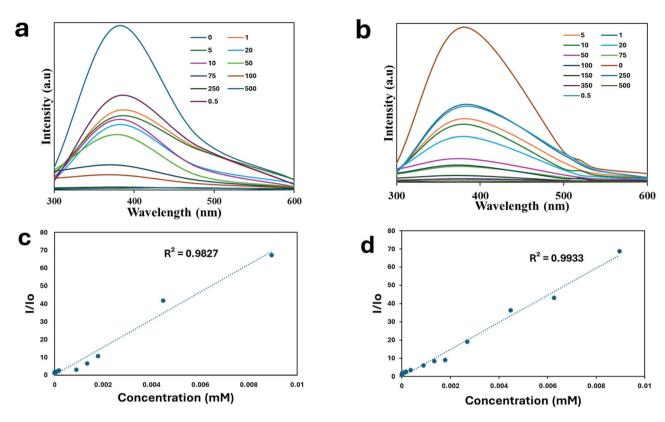
Fig. 7 (a) Photoluminescence spectra of various  $Fe^{2+}$  concentrations. (b) Photoluminescence spectra of different concentrations of  $Fe^{3+}$ . Stern–Volmer plot for (c)  $Fe^{2+}$ , and (d)  $Fe^{3+}$ .
