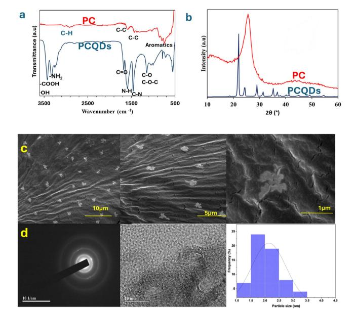
Fig. 1 (a) FTIR spectra of PCQDs and PC. (b) XRD spectra of PCQDs and PC. (c) SEM images of PCQDs. (d) SAED, TEM and particle size distribution curve of PCQDs.
