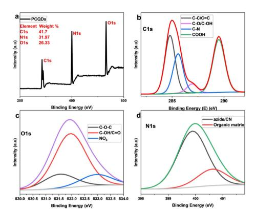
Fig. 3 (a) XPS survey spectrum of PCQDs. (b) C 1s XPS deconvolution. (c) O 1s XPS deconvolution. (d) N 1s XPS deconvolution.
