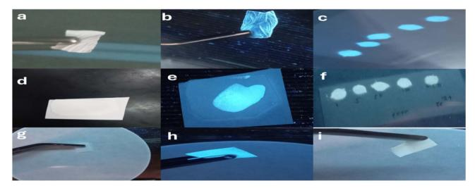
Fig. 8 (a) and (b) PVDF membrane before and after PCQD coating under UV-365 nm. (d) and (e) Invisible fingerprint under normal daylight and under UV-365 nm. (g)–(i) Filter paper before PCQD coating (UV-365 nm), after PCQD coating under UV-365 nm, and after adding 75 ppm of  $Fe^{3+}$  (UV-365 nm). (c) and (f) Filter paper coated with PCQDs and after adding  $Fe^{3+}$  at various concentrations under UV-365 nm.
