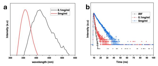
Fig. 5 (a) Emission spectra of PCQDs at various concentrations. (b) Time-resolved decay profiles of PCQDs at various concentrations
