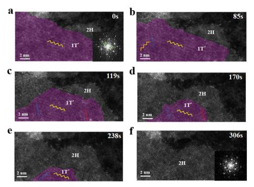
Fig. 4  $1T' \rightarrow 2H$  phase transition in monolayer MoS<sub>2</sub>. (a–f) Series of STEM-ADF images showing the  $1T' \rightarrow 2H$  phase transition as a function of time under electron beam irradiation. The insets are the corresponding FFT pattern.
