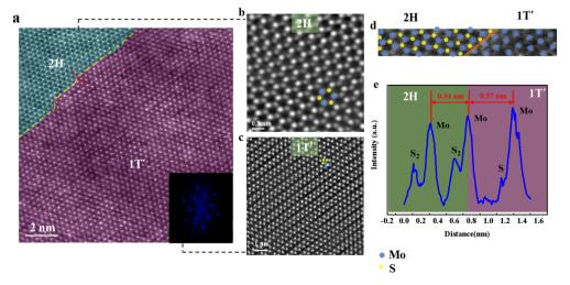
Fig. 2 (a) STEM-ADF image of an atomically thin phase boundary (indicated by the yellow dashed line) between the 2H and 1T' phase in a monolayer ce-MoS<sub>2</sub>. (b) STEM-ADF image of 2H phase of ce-MoS<sub>2</sub>. (c) STEM-ADF image of 1T' phase of ce-MoS<sub>2</sub>. (d) The enlarged STEM-ADF image at the 1T'/2H grain boundary. (e) Intensity line profile of the red dashed line in (a) confirming the 1T'/2H phase boundary.
