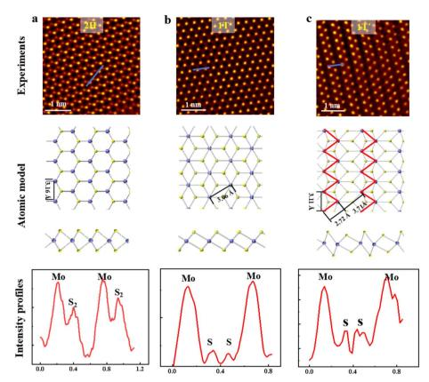
Fig. 1 Atomic-resolution STEM-ADF images of the monolayer MoS<sub>2</sub>: (a) 2H; (b) 1T; (c) 1T'. Corresponding atomic structures are shown in the lower panels. The intensity line profiles of each STEM-ADF from the blue lines are depicted below. Mo, blue; S, yellow.
