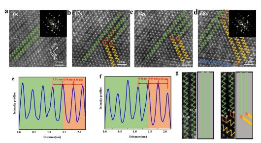
Fig. 3 (a-d) Series of STEM-ADF images showing the evolution of 1T' phase as a function of time under electron beam irradiation. The inset is the corresponding FFT pattern. (e and f) The intensity line profiles of each STEM-ADF from the red lines in (b). (g) The sequential ADF image of 1T' phase of changing the orientation diamond chains, scale bar 0.5 nm. The schemes on the right side represent the conduction channel before (green) and after (yellow) electron beam modulation.
