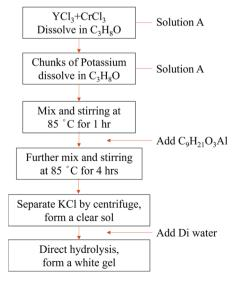
Fig. 1 Flow chart of sol-gel method.
