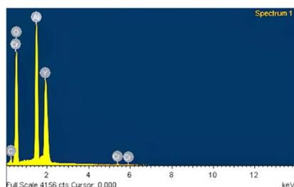
Fig. 7 EDS analysis of  $\text{Cr}^{4+}:\text{YAG}$  powder.
