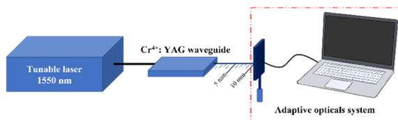
Fig. 10 Setup of the transmission characteristics measurement.
