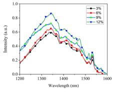
Fig. 8 Fluorescence spectra of Cr<sup>4+</sup>:YAG thin films with different doping concentrations.
