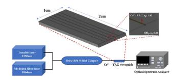
Fig. 9 Setup of the fluorescence characteristic measurement.
