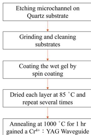
Fig. 2 Flow chart of thin film coating.
