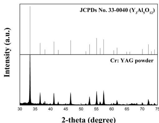
Fig. 5 XRD measurement of Cr<sup>4+</sup>:YAG powder with 3% doping concentration.
