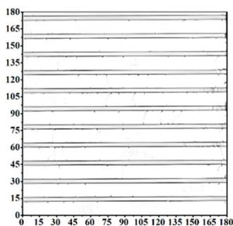
Fig. 3 OCT image of the surface structure of Cr<sup>4+</sup>:YAG waveguide.
