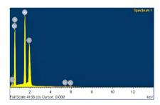
Fig. 7 EDS analysis of Cr<sup>4+</sup>:YAG powder.
