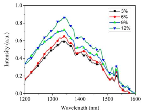
Fig. 8 Fluorescence spectra of  $\text{Cr}^{4+}:\text{YAG}$  thin films with different doping concentrations.
