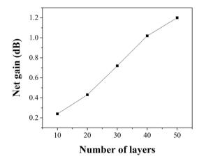
Fig. 16 The relationship between the number of thin-film layers and net gain.
