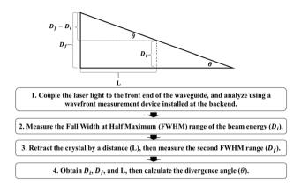
Fig. 12 Angle  $\alpha_{max}(\theta)$  calculation flow and schematic diagram.
