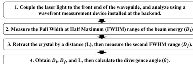
Fig. 12 Angle  $\alpha_{\max}(\theta)$  calculation flow and schematic diagram.
