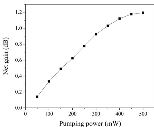
Fig. 15 Net gain as a function of pumping power of Cr<sup>4+</sup>:YAG thin films.
