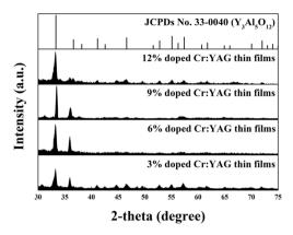
Fig. 6 Thin film diffraction pattern with different chromium doping concentrations.
