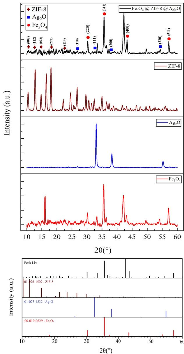
Fig. 3 XRD patterns of Fe<sub>3</sub>O<sub>4</sub>, Ag<sub>2</sub>O, and ZIF-8 nanoparticles, and the Fe<sub>3</sub>O<sub>4</sub>@ZIF-8@Ag<sub>2</sub>O nanocomposite.
