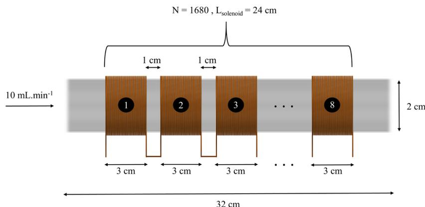
Fig. 2 Schematic of the designed solenoid wire coil.
