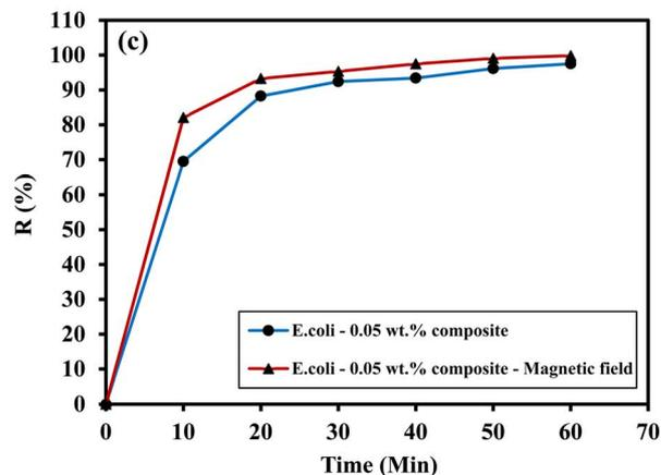
Fig. 6 Images of the magnetic reactor and trapped magnetic particles in the column (a). Effect of a magnetic field on the removal of *E. coli* concentrations versus different contact times; error bars indicate the standard deviation (b). Removal percentage of *E. coli* concentrations versus different contact times (c).
