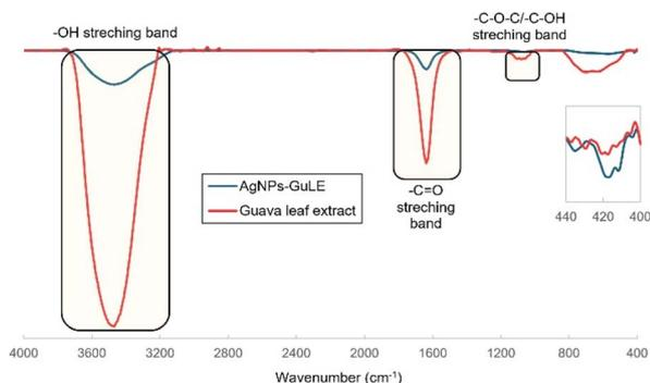
Fig. 6 FTIR spectra of the guava leaf extract (red) and the AgNPs-GuLE suspension.
