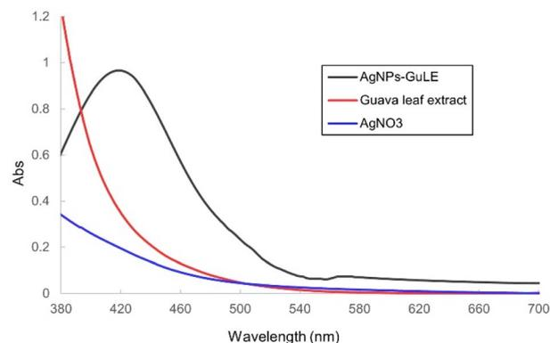
Fig. 1 Typical UV-vis spectra of AgNPs-GuLE, guava leaf extract, and AgNO<sub>3</sub>.
