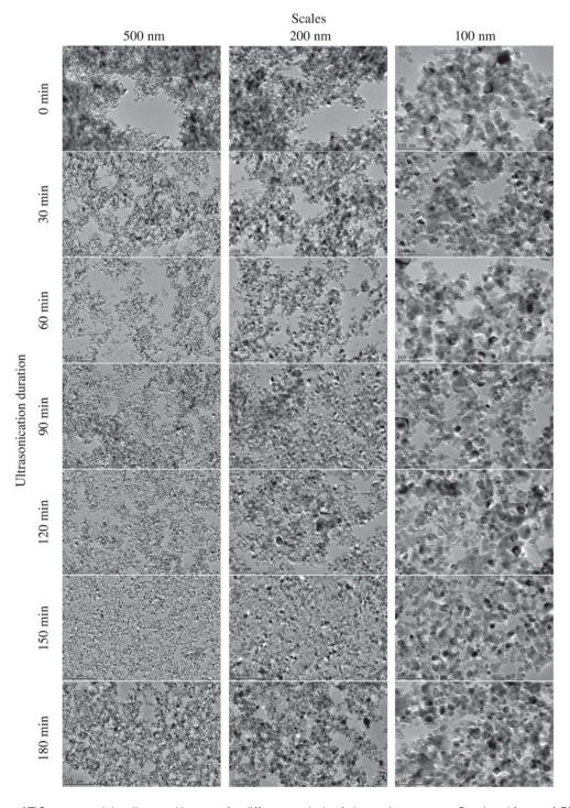
Fig. 4 TEM images of TiO<sub>2</sub> nanoparticles dispersed in water for different periods of ultrasonic treatment. Reprinted from ref. 39 with permission from Elsevier Ltd.
