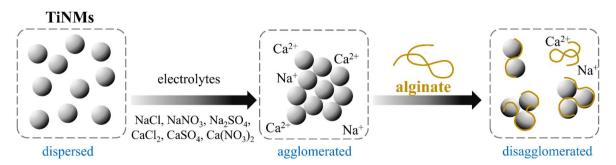
Fig. 8 Schematic presentation of disagglomeration and stabilization of TiO2 nanomaterials (TiNMs) by alginates. Adapted from ref. 166 with permission from Elsevier Ltd.
