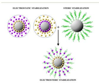
Fig. 3 Schematic representation of steric, electrostatic, and electrosteric stabilization of nanomaterials.
