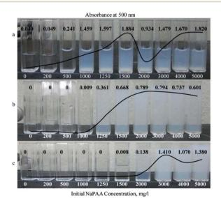
Fig. 6 Settling behaviour of  $TiO_2$  suspensions after 50 days of aging at different initial NaPAA concentrations: (a) 20 wt%, (b) 30 wt%, (c) 40 wt%. Reproduced from ref. 123 with permission from Elsevier Ltd.
