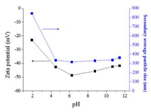
Fig. 7 Zeta potential and the secondary average particle size estimated by DLS in aqueous  $TiO_2$  dispersion (0.005 wt%) containing 0.01 wt% SHMP through supercritical  $CO_2$  (t=35 °C, p=1200 psi, saturation time 30 min). Reproduced with permission from ref. 38. Copyright under ACS AuthorChoice Licence.
