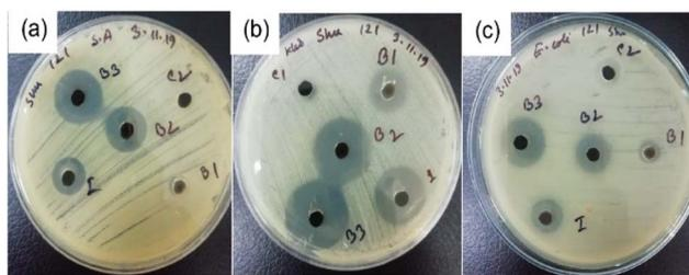
Fig. 14 Antibacterial study to determine the of inhibition zone by varying concentrations ( $B_1$ ,  $B_2$ ,  $B_3$ ) of PAM/NiO NC against (a) *S. aureus*, (b) *Klebsiella* spp. and (c) *E. coli* bacterial strains.
