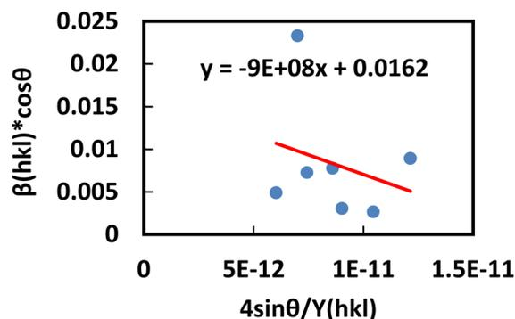
Fig. 6 Determination of the crystallite size of the synthesized PAM/NiO NC by UDM.
