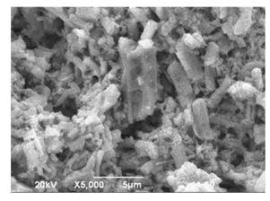
Fig. 13 SEM image of PAM/NiO NC at ×5000 magnification.
