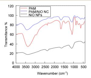
Fig. 3 FT-IR spectra of PAM/NiO NC & polyacrylamide.
