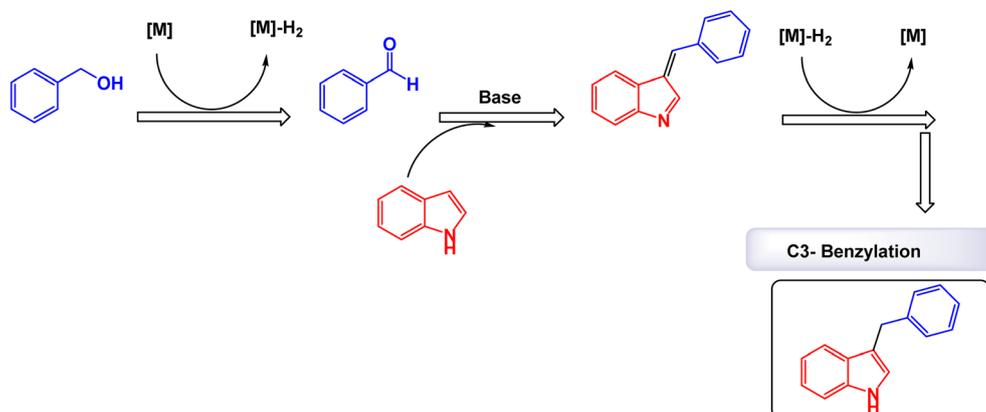
Scheme 37 Suggested mechanism for synthesis of 3-benzylated indoles [catalysis by MnFe<sub>2</sub>O<sub>4</sub> nanocomposite].
