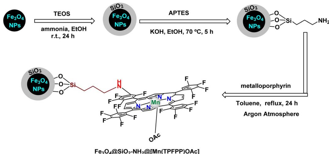
Scheme 1 General method to construct the  $\text{Fe}_3\text{O}_4@SiO_2-NH_2@[Mn(TPFPPOAc)]$  nanocomposite.
