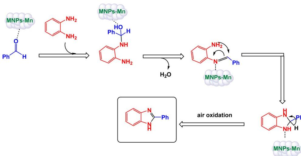
Scheme 22 Suggested mechanism for synthesis of benzimidazoles [catalysis by MnFe<sub>2</sub>O<sub>4</sub> nanocomposite].
