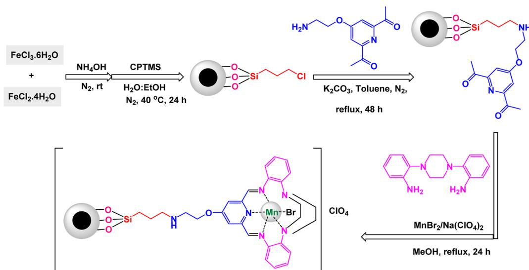
Scheme 23 General method for construction of  $[\text{Fe}_3\text{O}_4@\text{PAM-Schiff-base-Mn}][\text{ClO}_4]$  nanocomposite.
