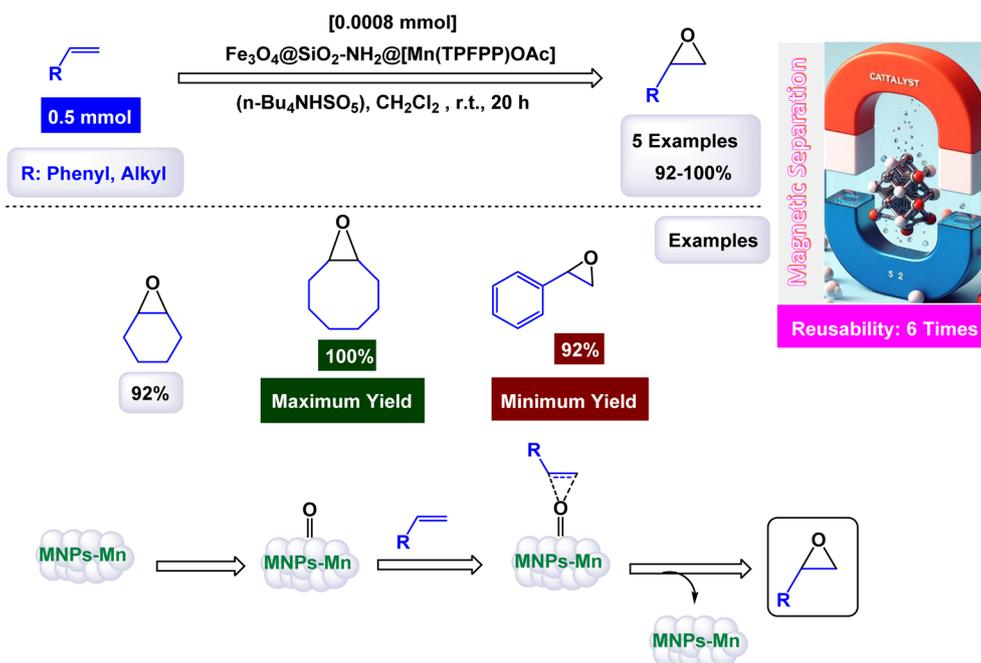
Scheme 2 Epoxidation of alkenes [catalysis by  $\text{Fe}_3\text{O}_4@SiO_2-NH_2@[Mn(TPFPPOAc)]$  nanocomposite].
