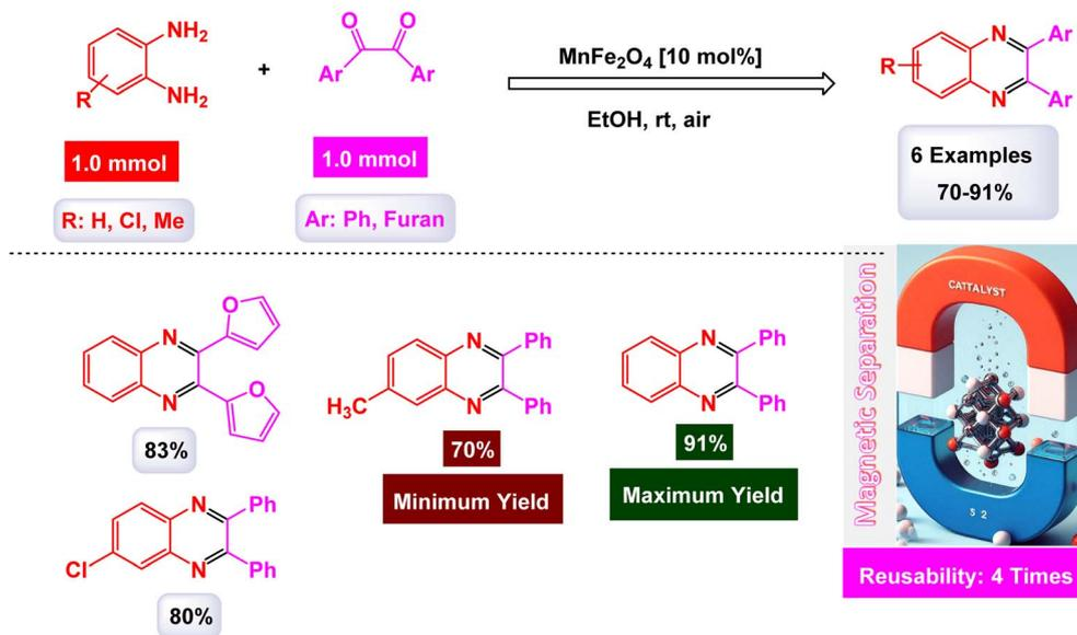
Scheme 21 Synthesis of quinoxalines [catalysis by MnFe<sub>2</sub>O<sub>4</sub> nanocomposite].
