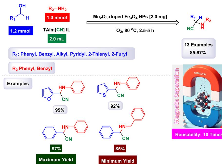
Scheme 34 Synthesis of alpha-aminonitriles from alcohols and amines [catalysis by Mn<sub>2</sub>O<sub>3</sub>-doped Fe<sub>3</sub>O<sub>4</sub> NPs nanocomposite].
