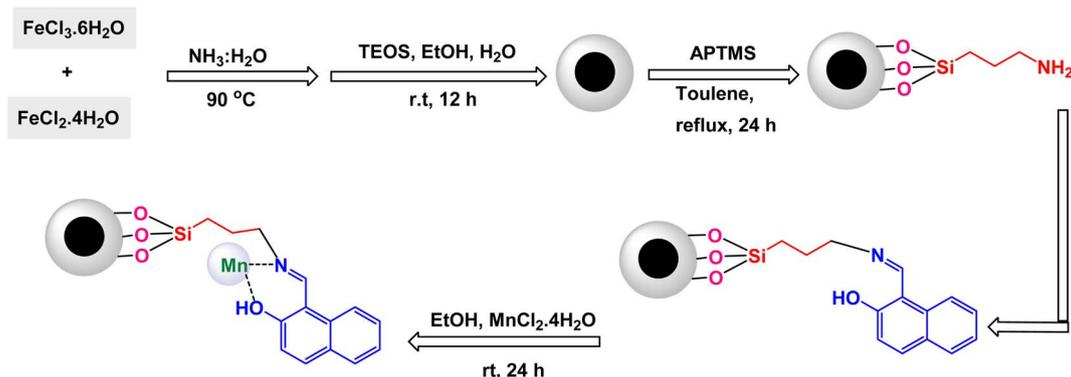
Scheme 26 General method for construction of  $\text{Fe}_3\text{O}_4@\text{SiO}_2@\text{Mn}$ -complex.
