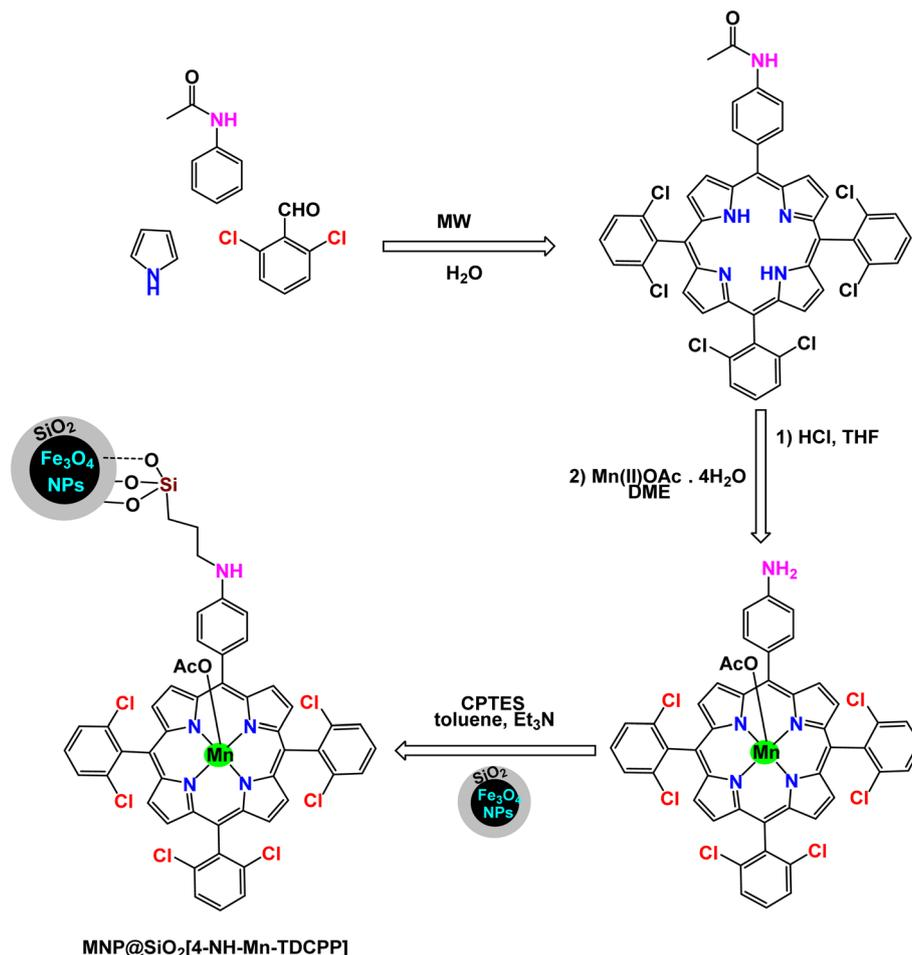
Scheme 3 General method to construct the MNP@SiO<sub>2</sub>[4-NH-Mn-TDCPP] nanocomposite.
