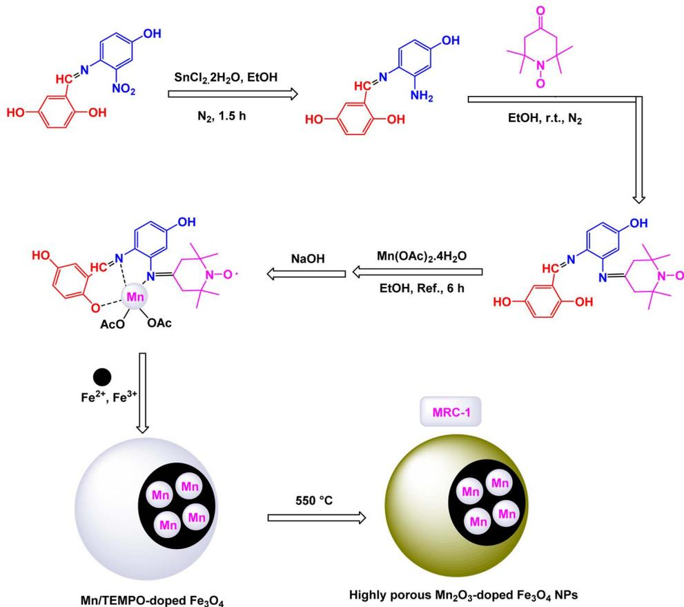
Scheme 33 General method to construct Mn<sub>2</sub>O<sub>3</sub>-doped Fe<sub>3</sub>O<sub>4</sub> NPs nanocomposite [MRC-1].
