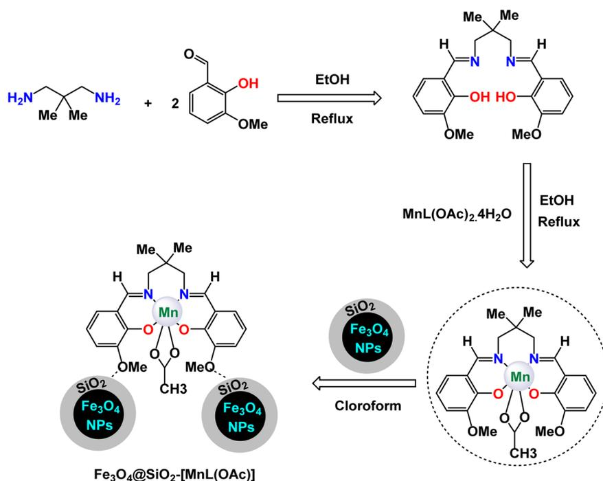
Scheme 7 General method to construct the  $\text{Fe}_3\text{O}_4@\text{SiO}_2\text{-}[\text{MnL}(\text{OAc})]$  nanocomposite.
