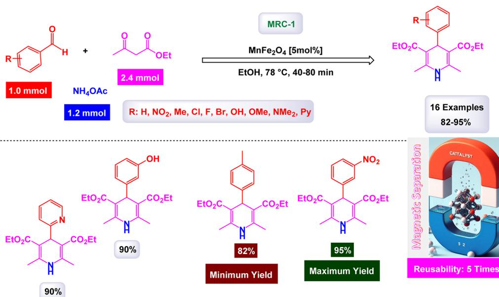
Scheme 29 Synthesis of 1,4-dihydropyridines [catalysis by  $\text{MnFe}_2\text{O}_4$  nanocomposite].
