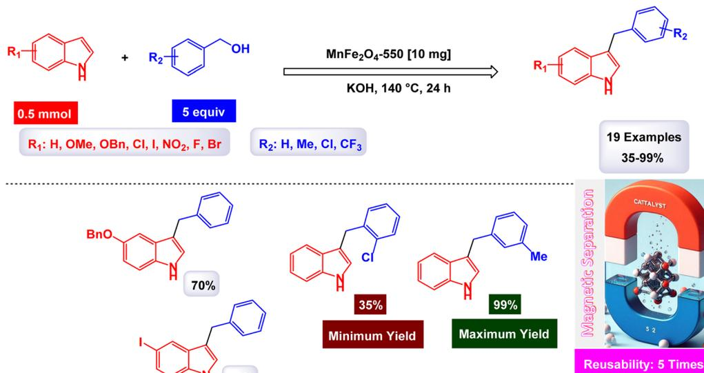
Scheme 36 Synthesis of 3-benzylated indoles [catalysis by MnFe<sub>2</sub>O<sub>4</sub> nanocomposite].
