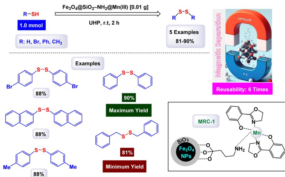
Scheme 13 Oxidation thiols to disulfides [catalysis by Fe<sub>3</sub>O<sub>4</sub>@SiO<sub>2</sub>-NH<sub>2</sub>@Mn(III) nanocomposite].
