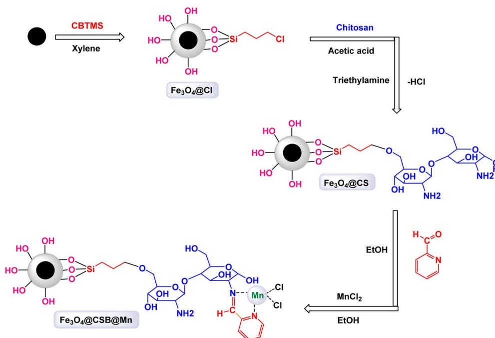
Scheme 30 General method for construction of  $\text{Fe}_3\text{O}_4@\text{CSBMn}$  nanocomposite.
