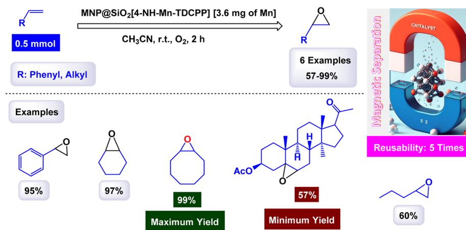
Scheme 4 Epoxidation of alkenes [catalysis by MNP@SiO<sub>2</sub>[4-NH-Mn-TDCPP] nanocomposite].
