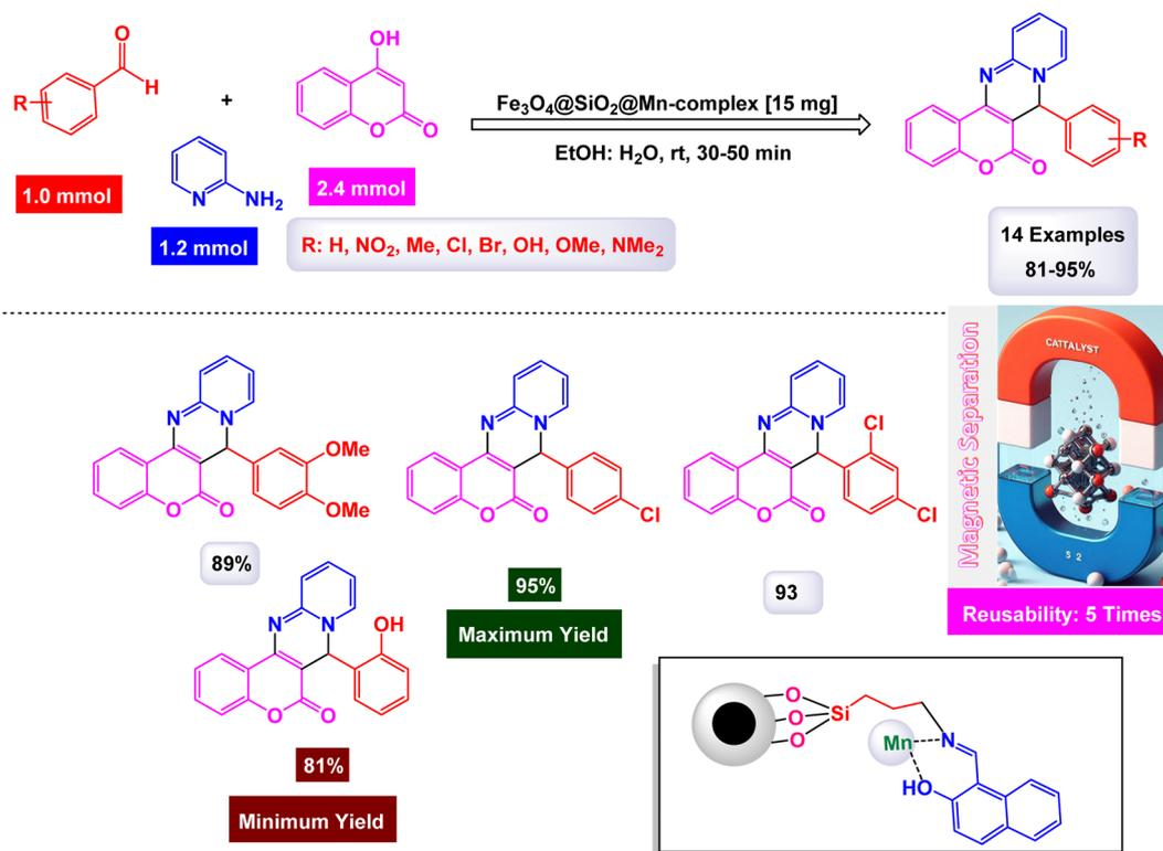
Scheme 27 Synthesis of 7-aryl[4,3-d]pyrido[1,2-a]pyrimidin-6(7H)-ones [catalysis by  $\text{Fe}_3\text{O}_4@\text{SiO}_2@\text{Mn}$  nanocomposite].
