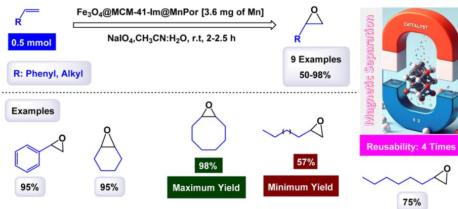
Scheme 6 Epoxidation of alkynes [catalysis by  $\text{Fe}_3\text{O}_4@\text{MCM-41-Im@mMnPor}$  nanocomposite].
