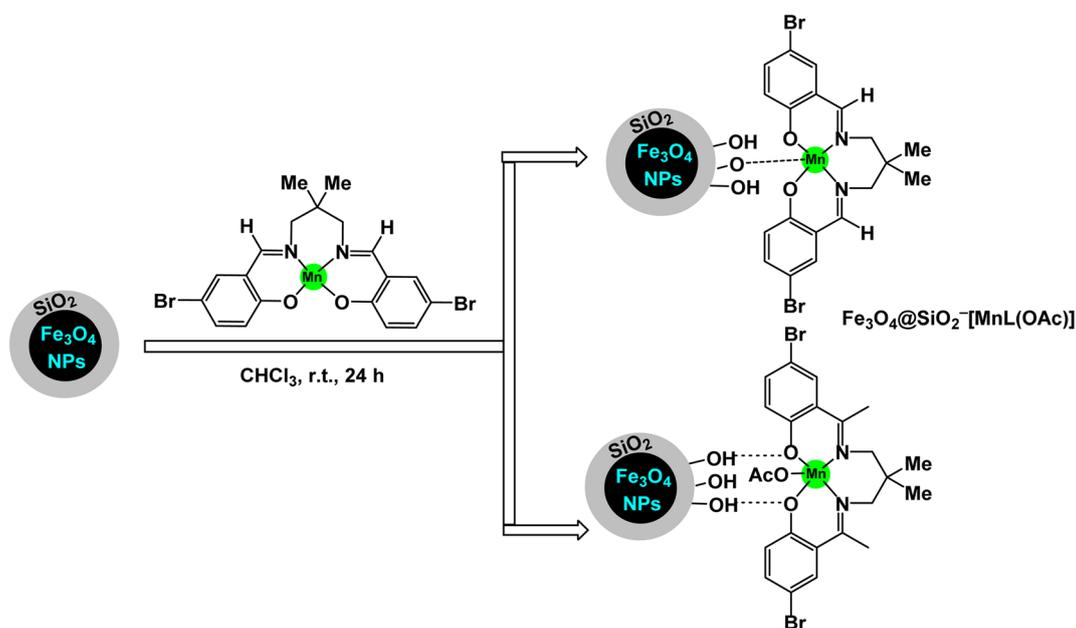
Scheme 10 General method to construct the  $\text{Fe}_3\text{O}_4@\text{SiO}_2\text{-[MnL(OAc)]}$  nanocomposite.
