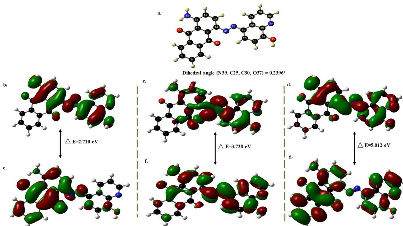
Fig. 6 (a). Optimized geometry of S9b; molecular orbitals of energy levels of (b). HOMO (c). HOMO+1 (d). HOMO+2 (e). LUMO (f). LUMO+1 (g). LUMO+2.
