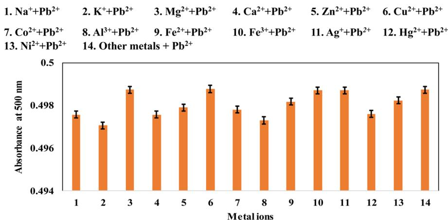
Fig. 5 Absorption changes of **S9b** (24.74  $\mu\text{g mL}^{-1}$ ) with Pb<sup>2+</sup> (5 equivalents) and metal ions (5 equivalents) in ethanol.
