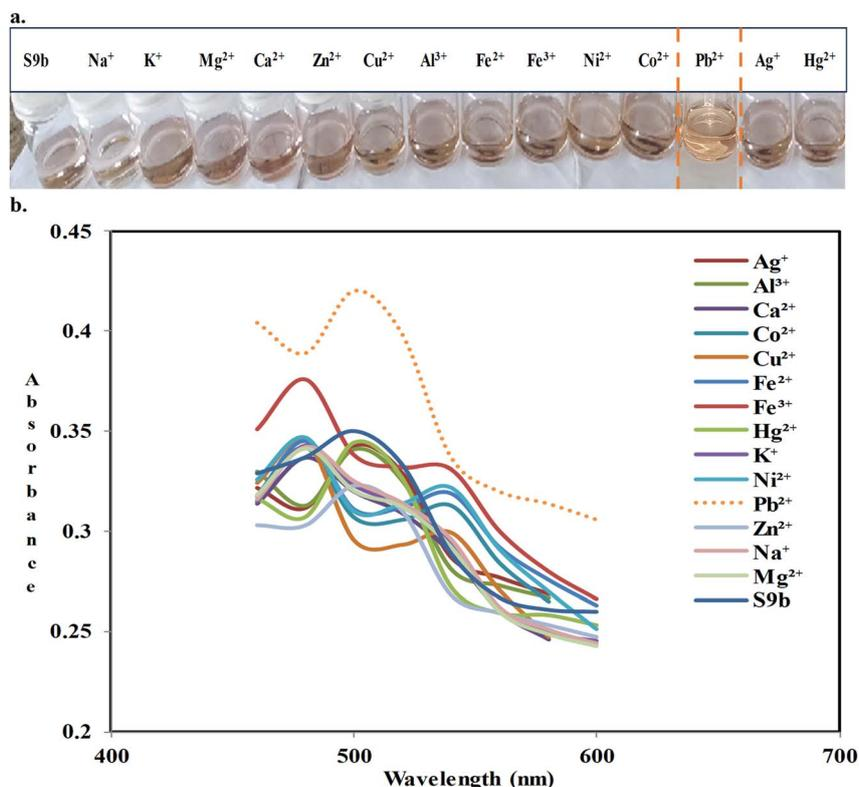
Fig. 1 Color changes of **S9b** in the presence of lead(II) ions and other cations in ethanol, pH 6 (a); overlaid spectra of **S9b** ( $0.9230 \text{ mg mL}^{-1}$ ) in the presence of five equivalents of each cation solution in ethanol (b).
