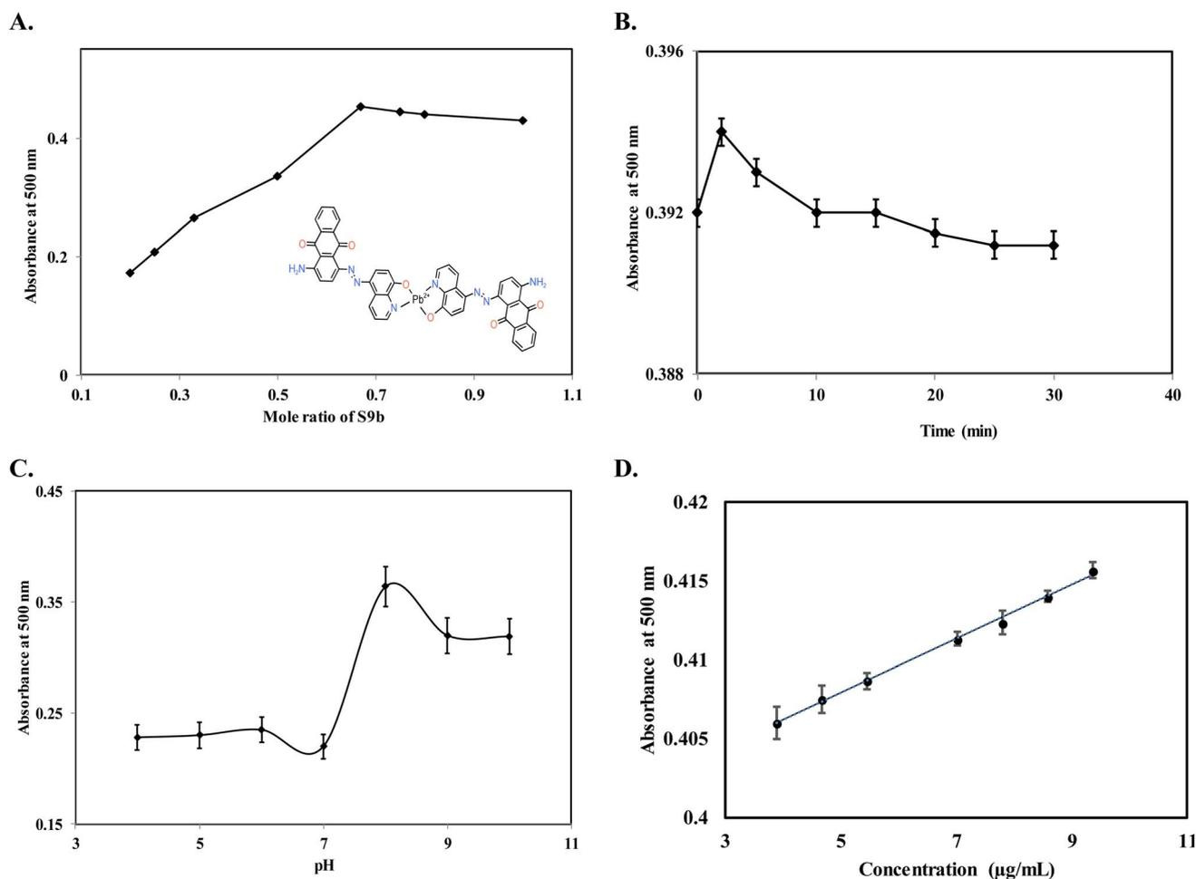
Fig. 2 Job's plot for **S9b** with  $\text{Pb}^{2+}$ . (Inset) Proposed structure of **S9b**- $\text{Pb}^{2+}$  (A); chelating time of reaction of **S9b** and  $\text{Pb}^{2+}$  (B); reaction pH between **S9b** and  $\text{Pb}^{2+}$  (C) and linear response of  $24.74 \mu\text{g mL}^{-1}$  **S9b** to varying concentrations of  $\text{Pb}^{2+}$  ( $3.90$ – $9.36 \mu\text{g mL}^{-1}$ ) in ethanol (D).
