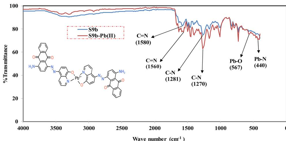
Fig. 3 Overlaid FTIR Spectra of **S9b** and **S9b**–Pb<sup>2+</sup>.
