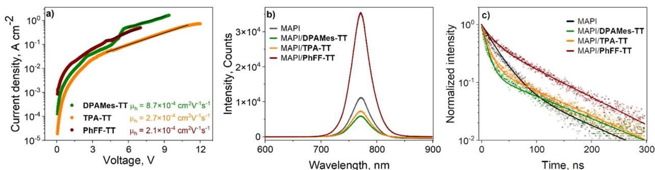
Fig. 4 (a) SCLC J–V Curves; (b) steady-state PL; (c) TRPL decay spectra, for perovskite/HTM bilayer films with **DPAMes-TT**, **TPA-TT**, **PhFF-TT**, and bare MAPbI<sub>3</sub> (MAPI).
