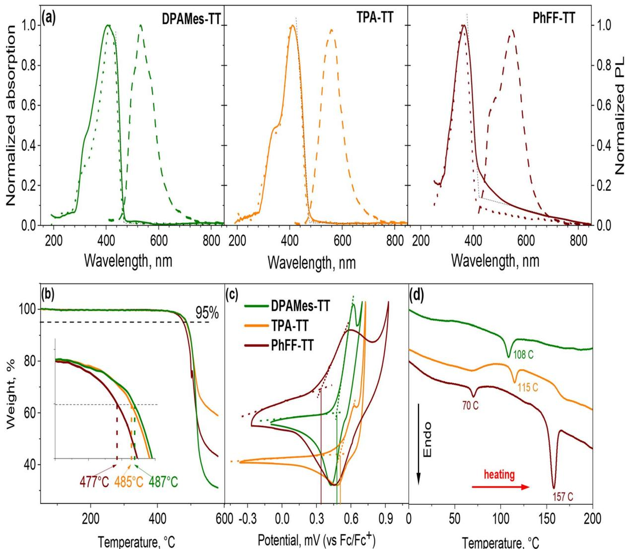
Fig. 2 (a) UV-visible absorption spectra of DPAMes-TT (green), TPA-TT (orange), and PhFF-TT (red) in dichloromethane solution (dotted lines) and in thin films (solid lines), and photoluminescence (PL) spectra in thin films (dashed lines); (b) TGA curves; (c) cyclic voltammetry (CV) curves; (d) differential scanning calorimetry (DSC) heating curves.
