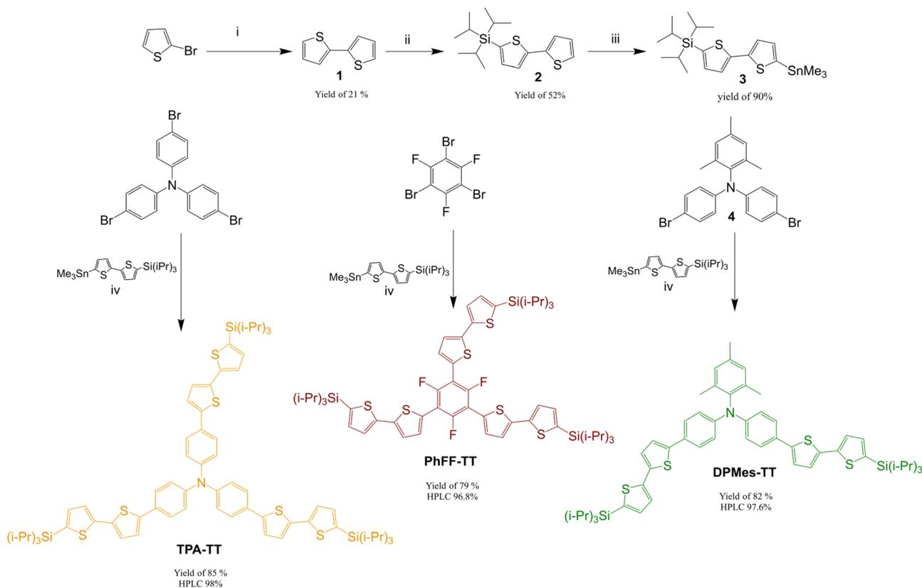
Fig. 1 Synthesis of small molecule HTMs. Conditions: i – THF, thiophen-2-yl magnesium bromide, Ni(dppp)Cl<sub>2</sub>; ii – THF, BuLi, (i-Pr)<sub>3</sub>SiCl; iii – THF, BuLi, Me<sub>3</sub>SnCl; iv – DMF, Pd(OAc)<sub>2</sub>, PPh<sub>3</sub>.
