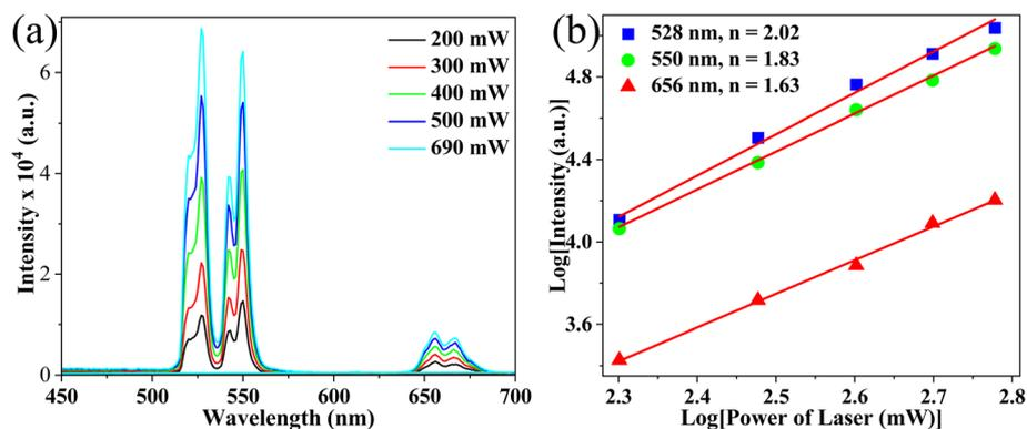
Fig. 9 Emission intensity-dependent power excitation of sample S2.
