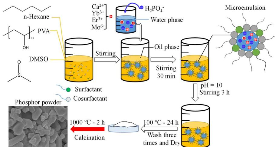
Fig. 1 The schematic synthesis of phosphors by microemulsion method.
